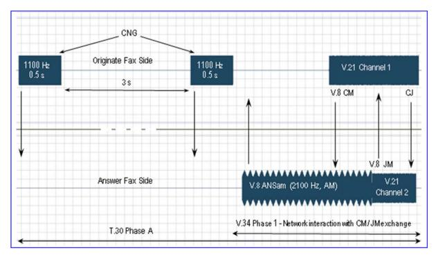
Figure 1: T.30 Phase A - V.34 Call Establishment
