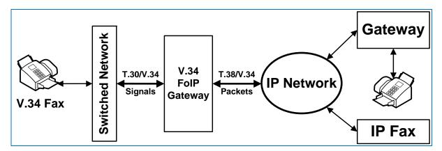
Figure 3: Typical layout of V.34 FoIP communication
