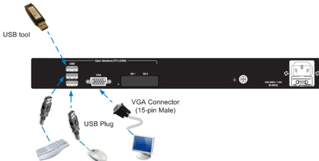
5. Power off and then power on the Mediant 800 to reboot the OSN server; the SBA Upgrade and Recovery process starts and logged messages are displayed on the VGA monitor.
