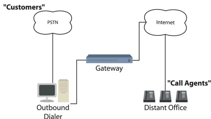
*Many use a media gateway to bridge a PSTN environment to a VoIP network. This design, though easy to implement, greatly increases the overall cost per channel of the system.*
