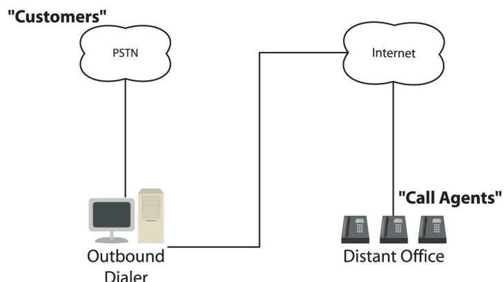
*Installing a PCI compatible media gateway preserves the original design of the outbound dialing system.*
