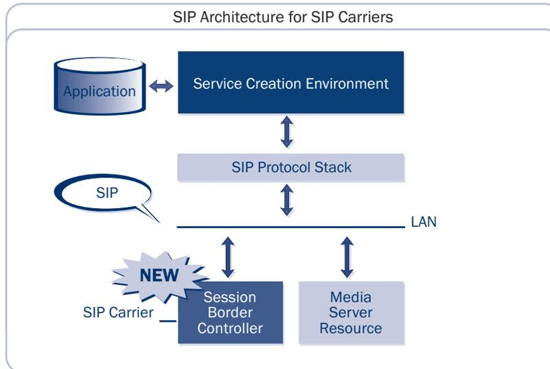
In deployments where a direct interface to a SIP carrier is available and there is no PSTN, the media gateway function is replaced with a Session Border Controller (SBC). The SBC provides important security and interoperability functions, including:
