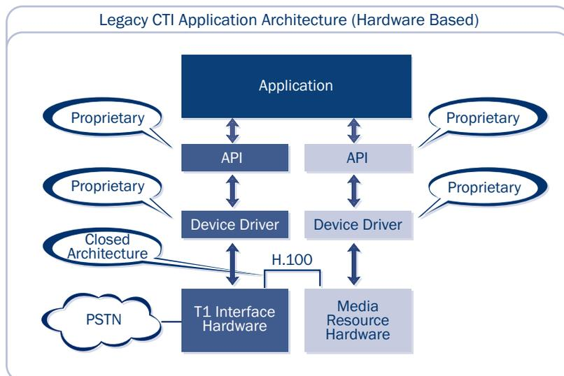
Most CTI applications support multiple DSP resource boards and/or interface boards as needed to connect to Loop Start, T1/E1, or Digital Station ports of enterprise or carrier TDM circuits. Solutions interconnect these different boards together with one of the popular TDM buses (H.100 or H.110).
