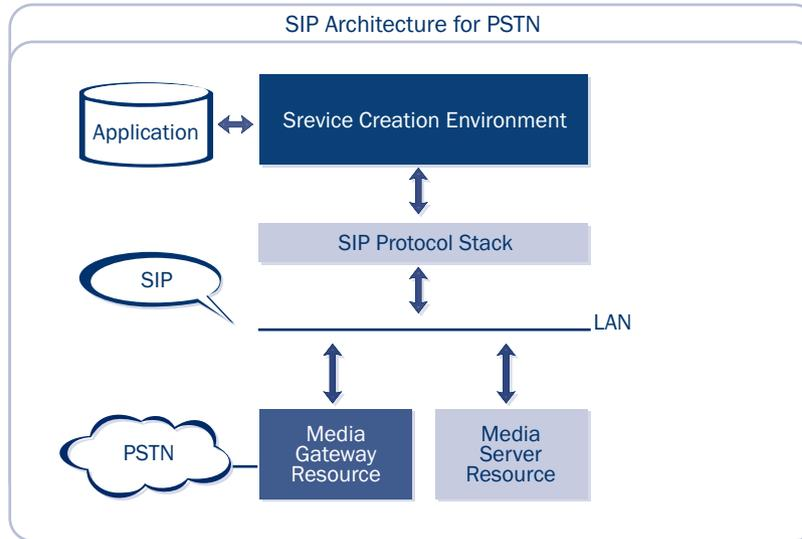
**Application/Service Creation Environment** – provides an environment for development and execution of the logic to be implemented by the completed application. Development tools include C/C++, Java, scripting languages, VoiceXML, CCXML and “drag and drop” graphical application environments.
