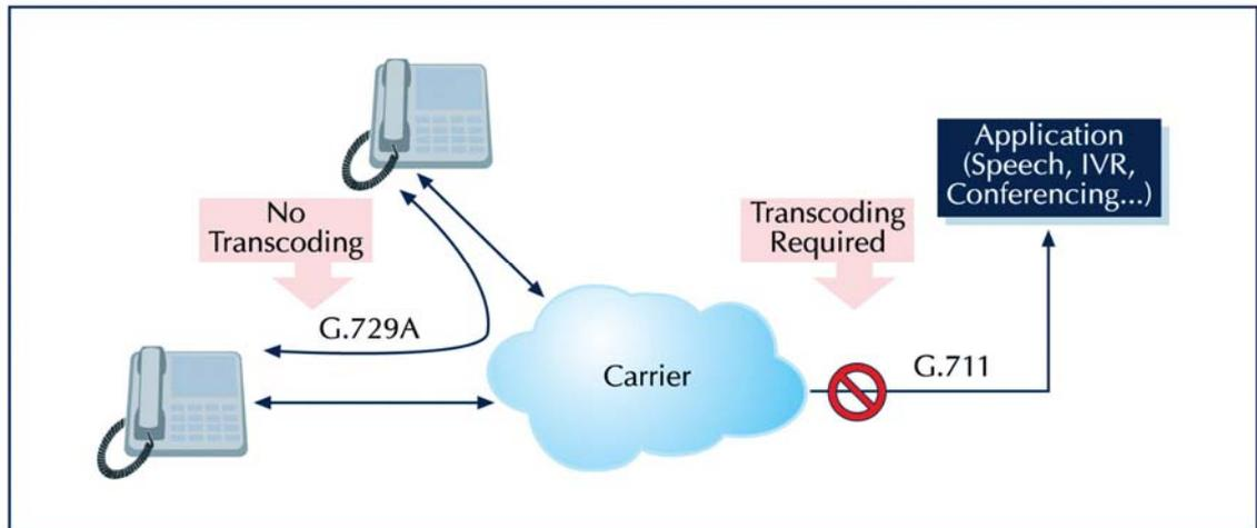
One might ask: "Does every conversation need transcoding?" The answer is "it depends", generally only the conversations that are interacting with the applications or different phone types need transcoding. Other end-to-end voice conversations between similar end points would not require transcoding and thus would use the LBR coder for the duration of the call.
