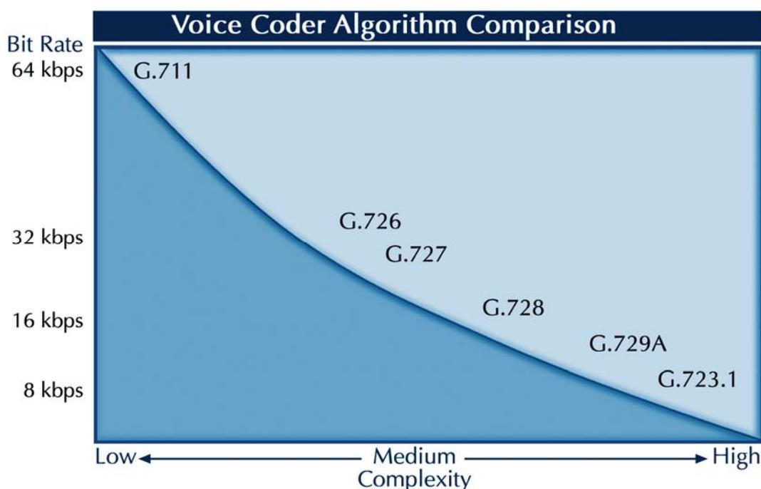
From uncompressed G.711 at 64 kbps to highly compressed G.723.1 at 5.3 kbps, the VoIP carriers could now choose the level of voice compression that would be applied to their customers.
