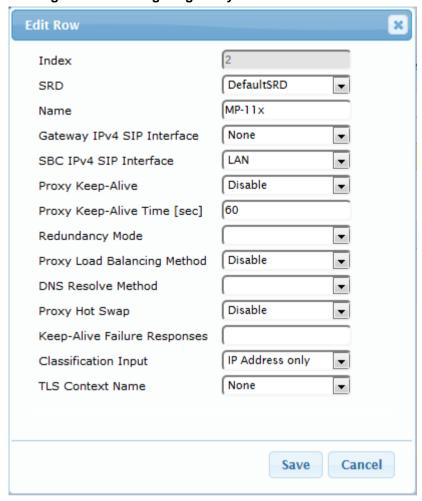
Figure 4-13: Configuring Proxy Set for Fax ATA device
