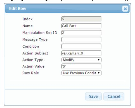
8. Configure another manipulation rule (Manipulation Set 4) for Flowroute SIP Trunk. This rule is applied to messages sent to the Flowroute SIP Trunk IP Group during Call Transfer initiated by the Skype for Business Server 2015 IP Group. This replaces the host part of the SIP Referred-By Header with the value, configured in the 'SIP Group Name' parameter for the Flowroute SIP Trunk IP Group.
