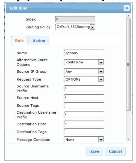
Figure 4-41: Configuring IP-to-IP Routing Rule for Terminating SIP OPTIONS – Rule Tab
