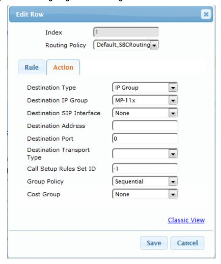
Figure 4-44: Configuring IP-to-IP Routing Rule for ITSP to Fax – Action tab
