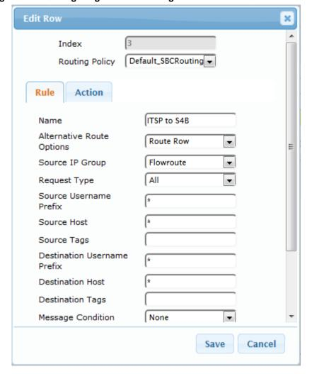
Figure 4-47: Configuring IP-to-IP Routing Rule for ITSP to S4B - Rule tab
