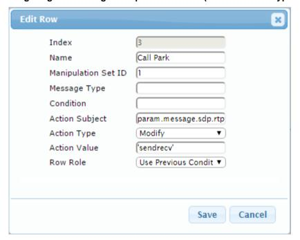
6. The following rule attempts to normalize the call processing state back to Skype for Business for the correct reply to the initially received "sendonly". For every SIP Re-INVITE message with the variable set to '1', change RTP mode to "recvonly". This SIP Re-INVITE message is the response sent from the Flowroute SIP Trunk to the Skype for Business initiated Hold.
