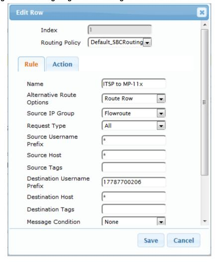
Figure 4-43: Configuring IP-to-IP Routing Rule for ITSP to Fax - Rule tab
