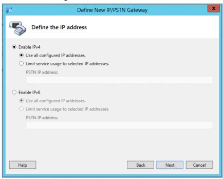
Define the listening mode (IPv4 or IPv6) of the IP address of your new PSTN gateway, and then click Next. 8. Define a *root trunk* for the PSTN gateway. A trunk is a logical connection between the Mediation Server and a gateway uniquely identified by the following combination: Mediation Server FQDN, Mediation Server listening port (TLS or TCP), gateway IP and FQDN, and gateway listening port.
