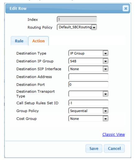
Figure 4-48: Configuring IP-to-IP Routing Rule for ITSP to S4B - Action tab
