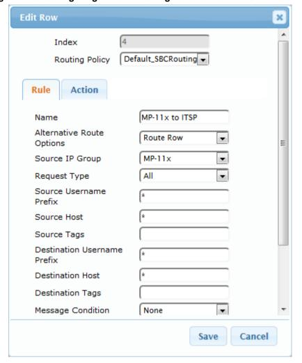
Figure 4-49: Configuring IP-to-IP Routing Rule for Fax to ITSP - Rule tab
