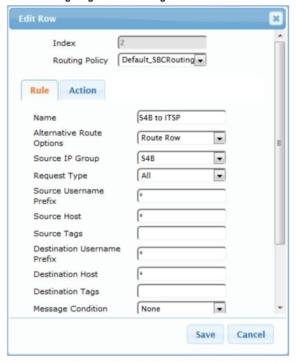
Figure 4-45: Configuring IP-to-IP Routing Rule for S4B to ITSP - Rule tab
