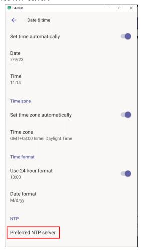
Admins can alternatively use the newly added parameter date\_time/ntp/server\_address in the phone's .cfg configuration file.
