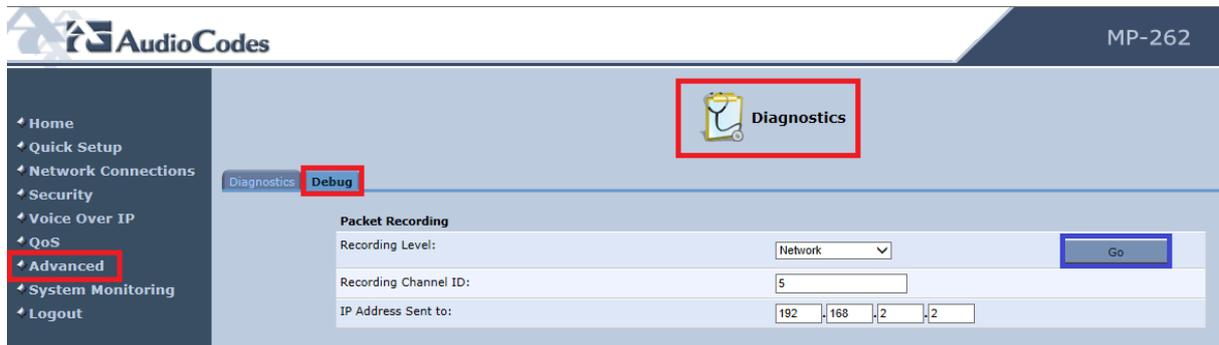
The screenshot shows the AudioCodes MP-262 web interface. The left sidebar contains a navigation menu with 'Advanced' highlighted. The main content area shows the 'Diagnostics' section, with 'Debug' selected. Under 'Packet Recording', the following fields are visible:
