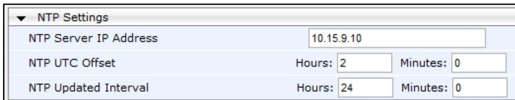
2. Set the **NTP Server IP Address** to <NTP Server IP-Address> (e.g., 10.15.9.10).
