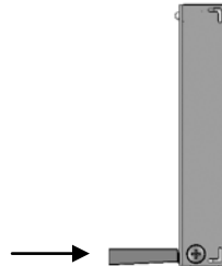
Figure 6-3: Module Handle Pushed In (Top View)
