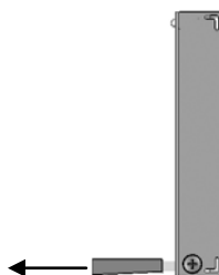
Figure 6-2: Module Handle Partially Pulled Out (Top View)
