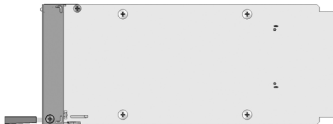
Figure 6-4: Extracted Blank AMC Module (Top View)
