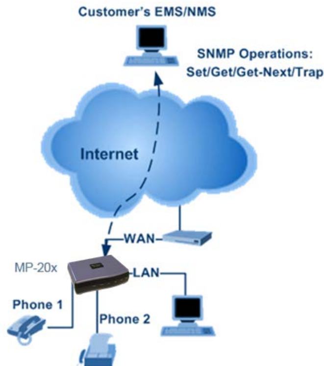
Figure 14-12: SNMP Network Architecture
