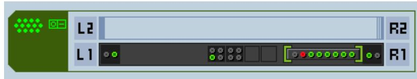
The Mediant 2000 Status pane graphically represents the status of the one or two-module device. If one of the modules fails, the status of the Mediant 2000 is indicated as failed. The Mediant 2000 Status pane indicates trunk status: Green for enabled, red for disabled and gray for locked (manually out of service) mode.
