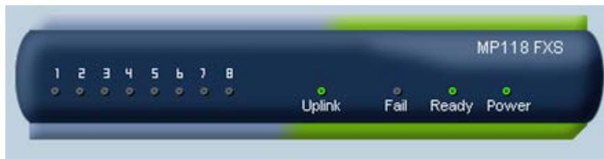
The Status pane represents MediaPacks and their LEDs indicating channel status (green- for off-hook and gray- for on-hook), LAN and Ready LEDs (refer to the table below). Data and Control LEDs are not represented and are always colored in *gray*.
