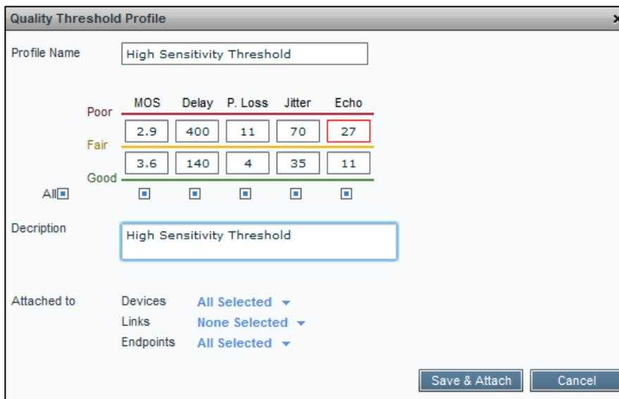
6. Click the **Attach** button; the profile is displayed in the QoE Thresholds screen.
