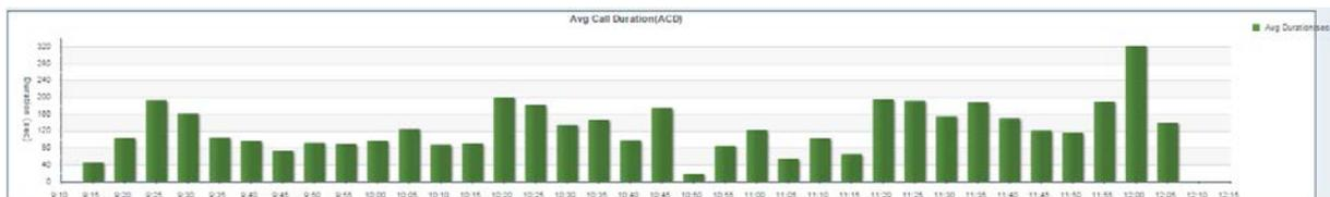
The chart helps you assess calls performance at a glance. The chart shows when the ACDs were longest compared to when shortest. You can compare this to Successful/Failed Calls, Failed Rate, Call Quality, Utilization, MOS, Packet Loss, Jitter, Delay or Echo charts, to identify correlation and make a diagnosis.
