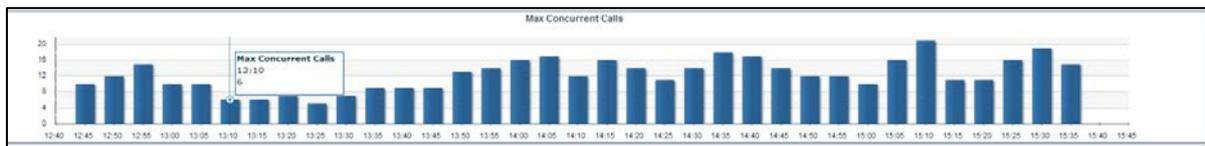
The chart helps you assess calls performance at a glance. The chart shows when the maximum concurrent calls *peaked* compared to when they *dipped*. You can compare this to Successful/Failed Calls, Average Call Duration, Failed Rate, Call Quality, Utilization, MOS, Packet Loss, Jitter, Delay and/or Echo charts, to identify correlation and make a diagnosis.
