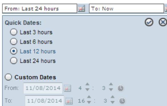
2. Under 'Quick Dates', select a time range and click
