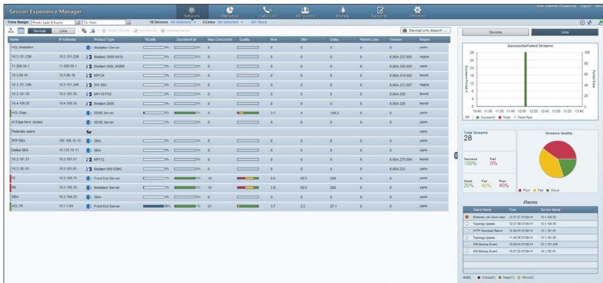
Columns show each device's share of calls as a percentage, ASR (average success rate), Quality distribution, MOS, Jitter, Delay and Packet Loss, allowing you access to specific information and consequently enhancing management efficiency.
