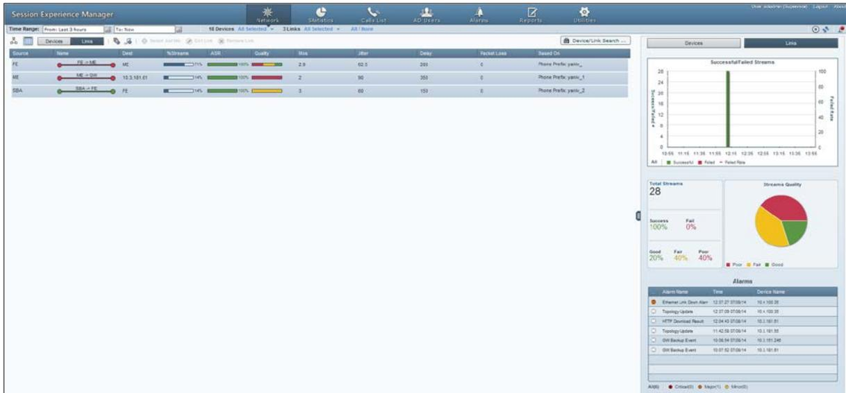
Columns show each link's Source, Name, Destination, %Streams, ASR, Quality, MOS, Jitter, Delay, Packet Loss, Version, and Region, allowing you access to specific information and consequently enhancing management efficiency.
