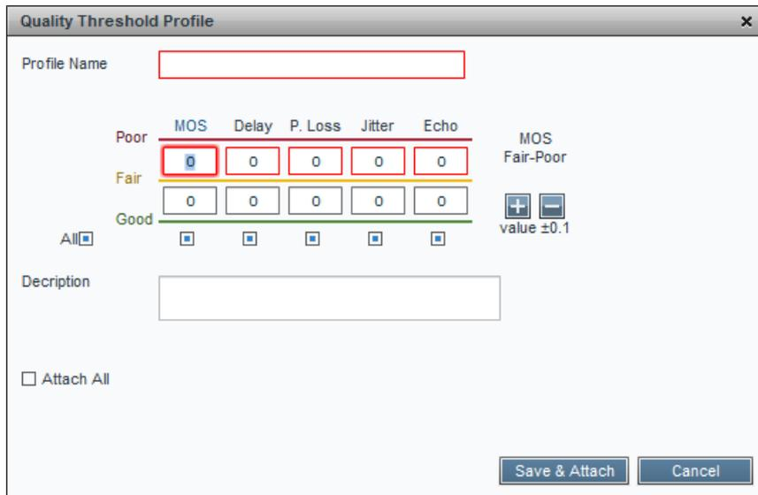
4. Click the **+** or the **-** until the threshold value you require is displayed. Each click increments or decreases the threshold by **0.1 (MOS, Packet Loss)**, or by **1 (Delay, Jitter, Echo)**. Alternatively, enter the value you require.
