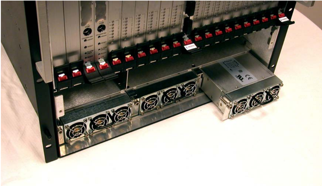
Figure 45-5: Removing the PS from the Chassis
