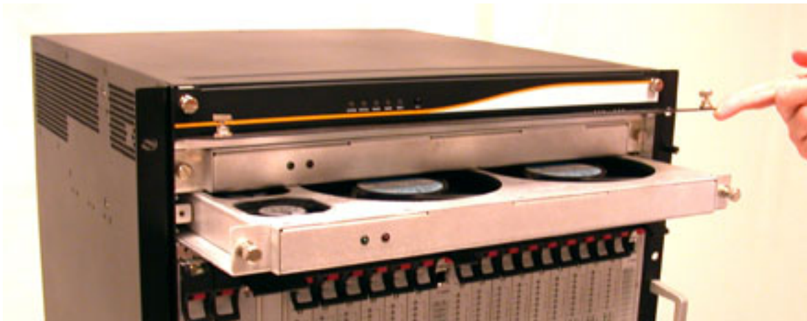
Figure 45-8: Replacing the Fan Tray Unit
