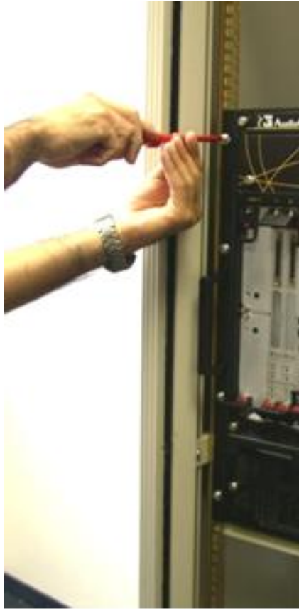
Figure 16-1: Attaching the Chassis to the Rack
