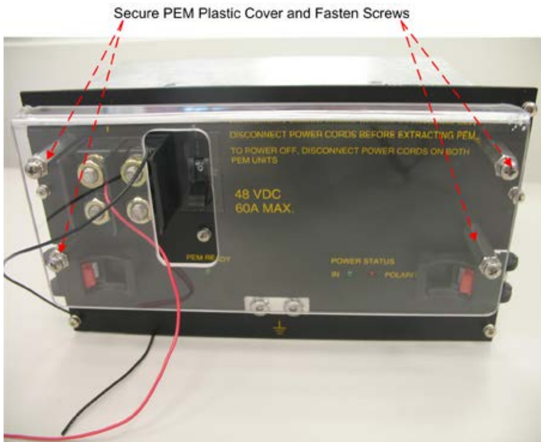
Figure 16-5: Secure the PEM Plastic Cover Screws
