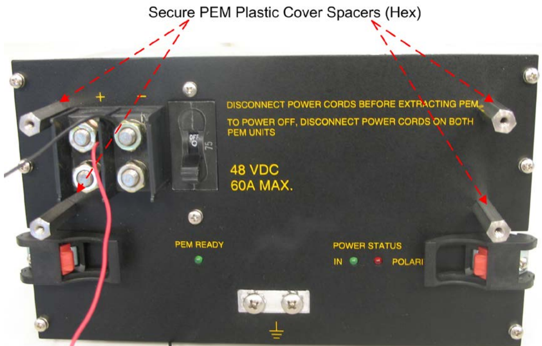
Figure 16-4: Securing the PEM Plastic Cover Spacers (Hex)
