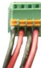
Figure 5-20: Wires Inserted in Terminal Block
