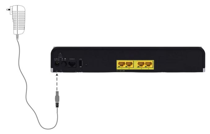
4. Switch on the device by pressing-in the power button located on the rear panel. When the device receives power, the **Power** LED turns on (green).
