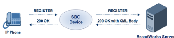
Figure 28-5: Interoperability with BroadWorks Registration Process
