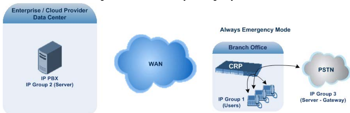
Figure 30-2: CRP in Always Emergency Mode
