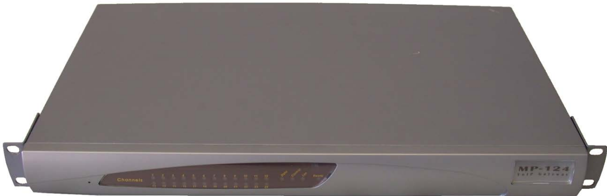
Figure 4-2: Attached Brackets for Rack Installation
