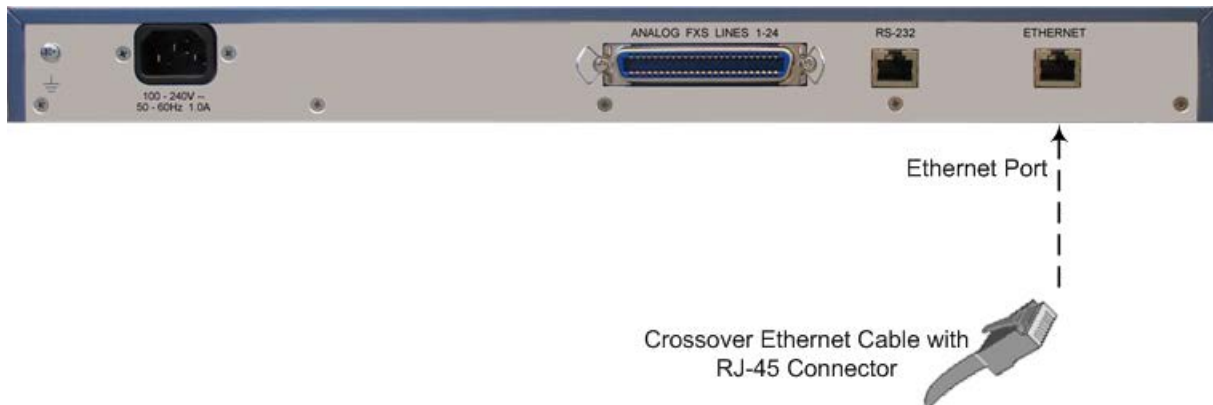
Figure 5-6: Connecting MP-124 to the Ethernet (e.g., Rev. E model)
