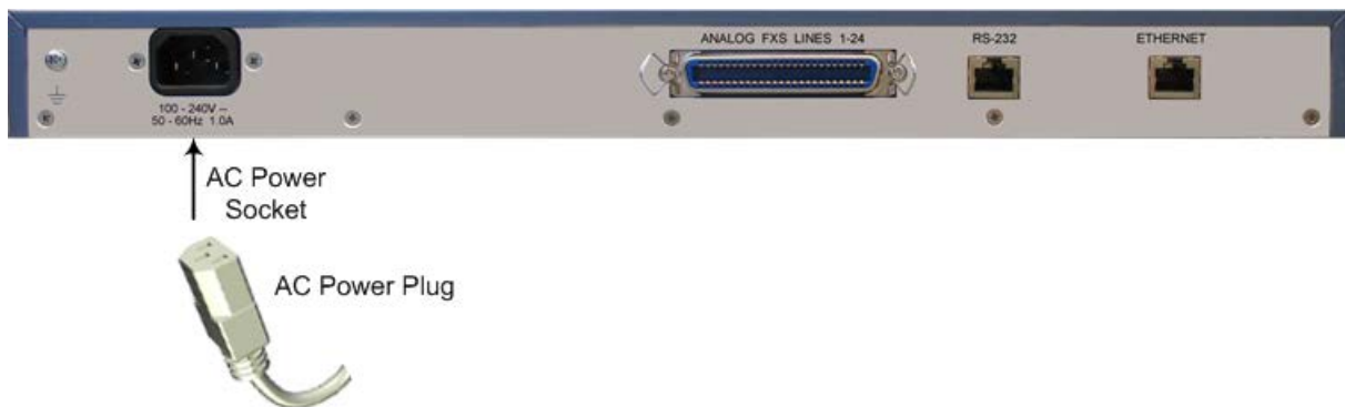
Figure 5-29: Connecting MP-124 to AC Power Supply (e.g., Rev. E model)
