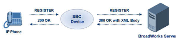
Figure 28-5: Interoperability with BroadWorks Registration Process
