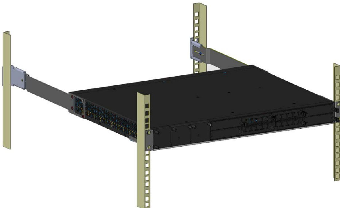
Figure 4-11: Front-Mounting Brackets Flush and Aligned with Front-Rack Posts (> 70 cm)
