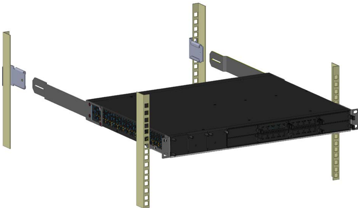
Figure 4-7: Sliding Rear-Mounting Flanges into the Rear-Mounting Brackets (> 70 cm)
