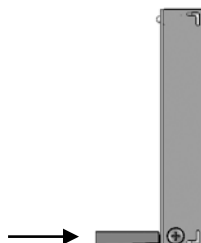
Figure 6-3: Module Handle Pushed In (Top View)
