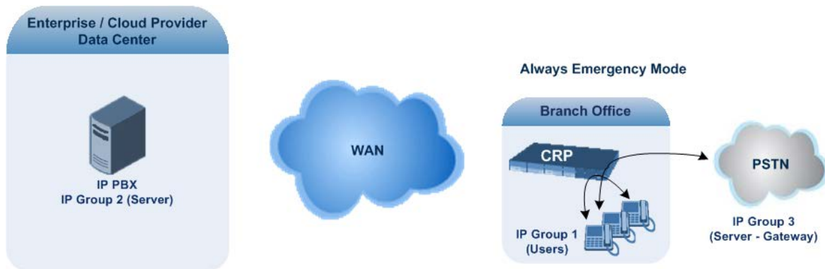
Figure 31-2: CRP in Always Emergency Mode
