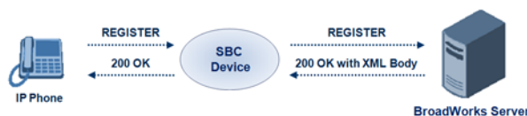
Figure 29-5: Interoperability with BroadWorks Registration Process
