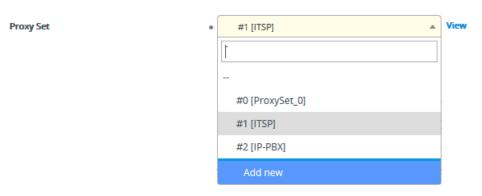
The table (e.g., IP Groups table) and dialog box in which the **Add new** option was selected is minimized to the bottom-left corner of the Web interface and a dialog box appears for adding a new row in the referenced-table (e.g., Proxy Sets table).
