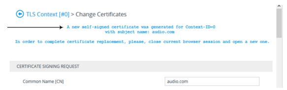
8. Save the configuration with a device reset for the new certificate to take effect.
