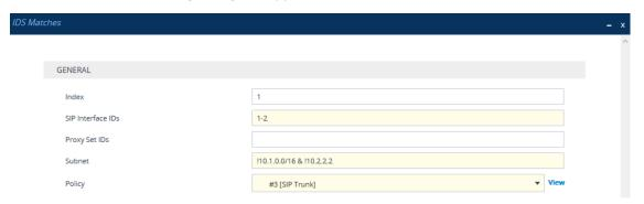
The figure above shows a configuration example where the IDS Policy "SIP Trunk" is applied to SIP Interfaces 1 and 2, and to all source IP addresses outside of subnet 10.1.0.0/16 and IP address 10.2.2.2.
