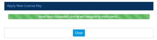
7. Clock Close to close the message box; you are logged out of the Web interface and prompted to log in again. The features and capabilities displayed on the License Key page now reflect the newly installed License Key.
