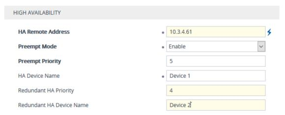
b. In the 'HA Remote Address' field, enter the Maintenance IP address of the second device.
