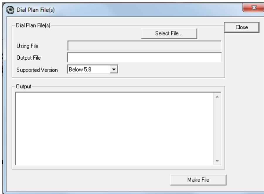
4. Click the **Select File** button, navigate to the desired folder, and then select the file to be converted; the selected file name (but with the *.dat* extension) and path is displayed in the 'Output File' field. The output file name may be altered.
