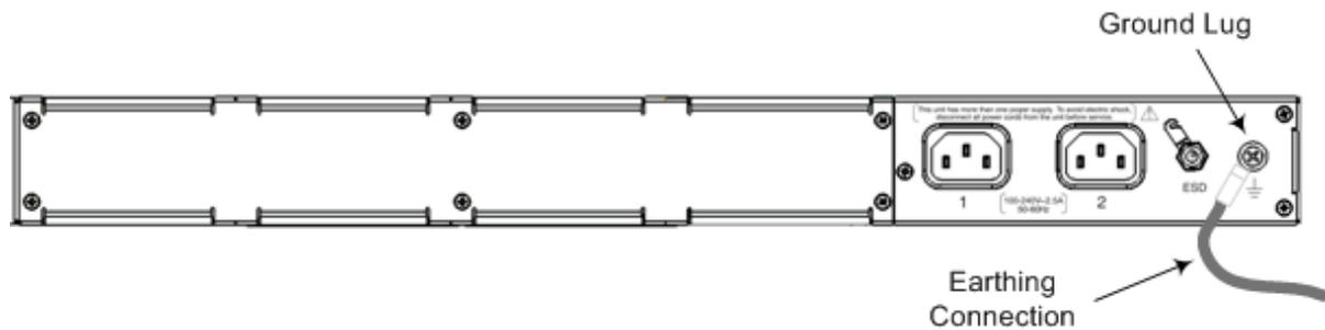
2. Connect the other end of the strap to a protective earthing. This should be in accordance with the regulations enforced in the country in which the device is installed.
