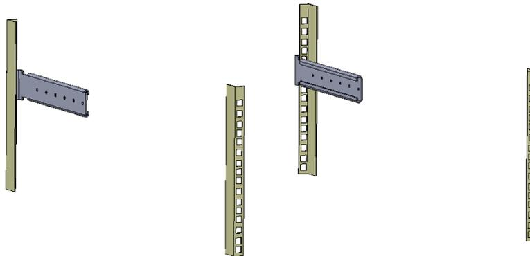
3. Attach the rear-mounting flanges to the rear sides of the chassis, using three screws (supplied) per flange.
