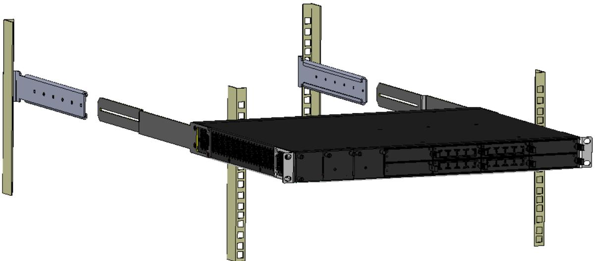
6. Hold the chassis in position while the second person secures the rear-mounting flanges to the rear-mounting brackets. Insert the supplied screws (6-32 x 5/16 inch) from the inside of the rack, through the flange's grid and into the screw hole on the rear-mounting bracket. Finger-tighten the screws but make sure that the screws are **NOT fully tightened** and that the flange can freely move on the slide rails of the rear-mounting bracket.
