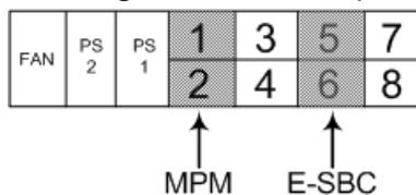
5. Push the module handle of the MPM until it clicks firmly in to engage the MPM with the chassis backplane.
