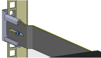
**Figure 4-9: Fastening Rear-Mounting Flange to Rear-Mounting Bracket (> 70 cm)**
