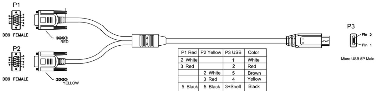
➤ **To connect the serial interface port to a computer:**
