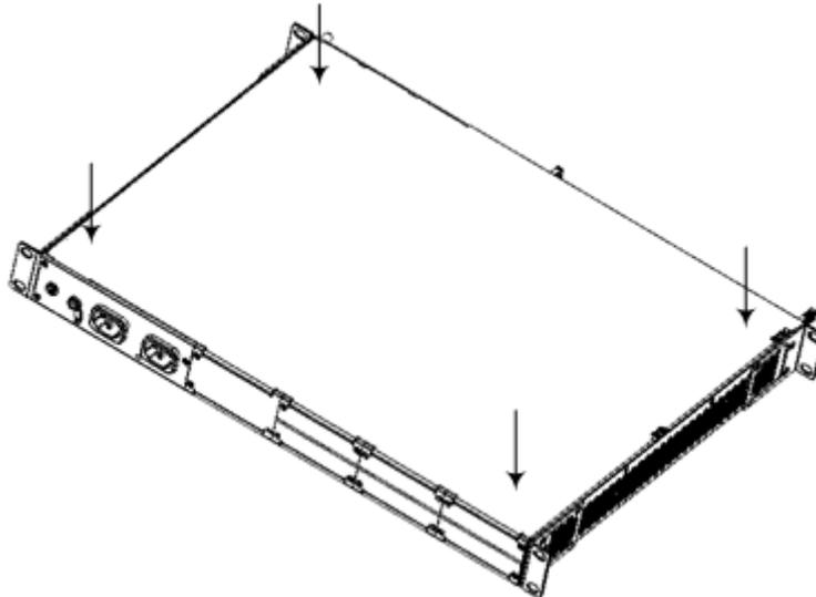
3. Peel off the adhesive, anti-slide rubber feet (supplied) and stick one in each anti-slide groove.
