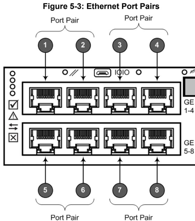
It is important that the two ports in the Ethernet Group making up a pair are connected to different switches (but in the same subnet). The figure below illustrates an example of implementing Ethernet-port redundancy:
