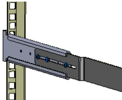
7. Hold the chassis for support while the second person positions the chassis so that the front-mounting brackets are flush against the front-rack posts and that the holes of the front-mounting brackets align with the holes on the front-rack posts.
