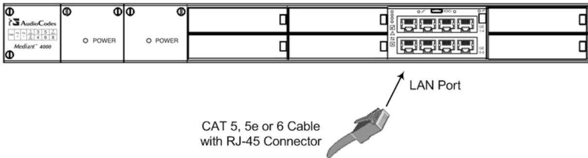
2. Connect the other end of the cable to the LAN network.
