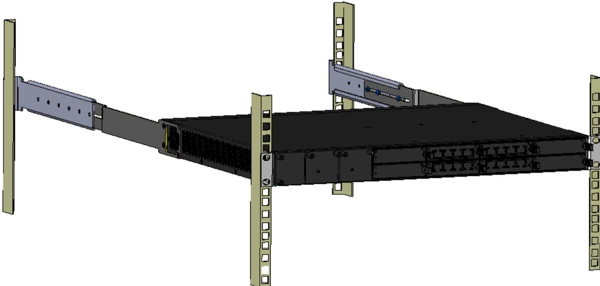
8. Hold the chassis in position while the second person secures the two front-mounting brackets to the front posts, by finger-tightening 19-inch rack bolts (not supplied) to the rack posts.
