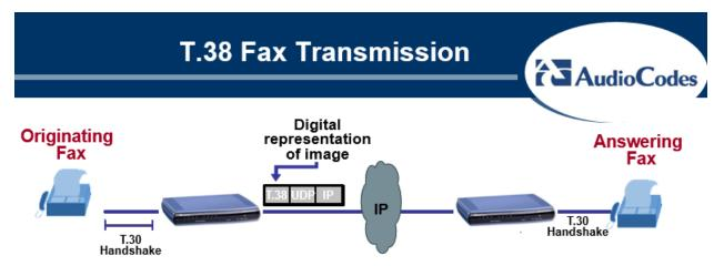
T.38 is an ITU recommendation for sending fax messages over IP networks in real time by encapsulating a standard G3 fax data stream.
