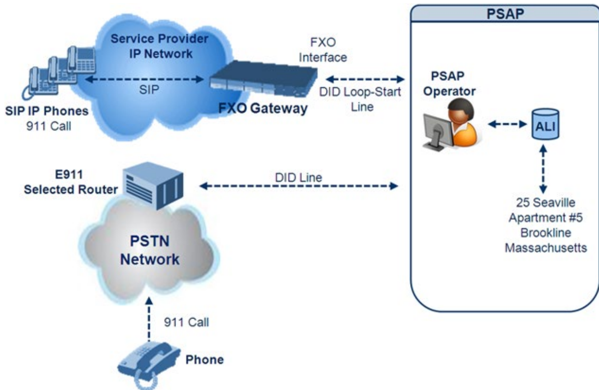
Figure 29-4: FXO Device Interfacing between E911 Switch and PSAP
