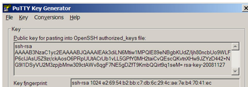
Figure 33-10: PuTTY Key Generator-Public Key
