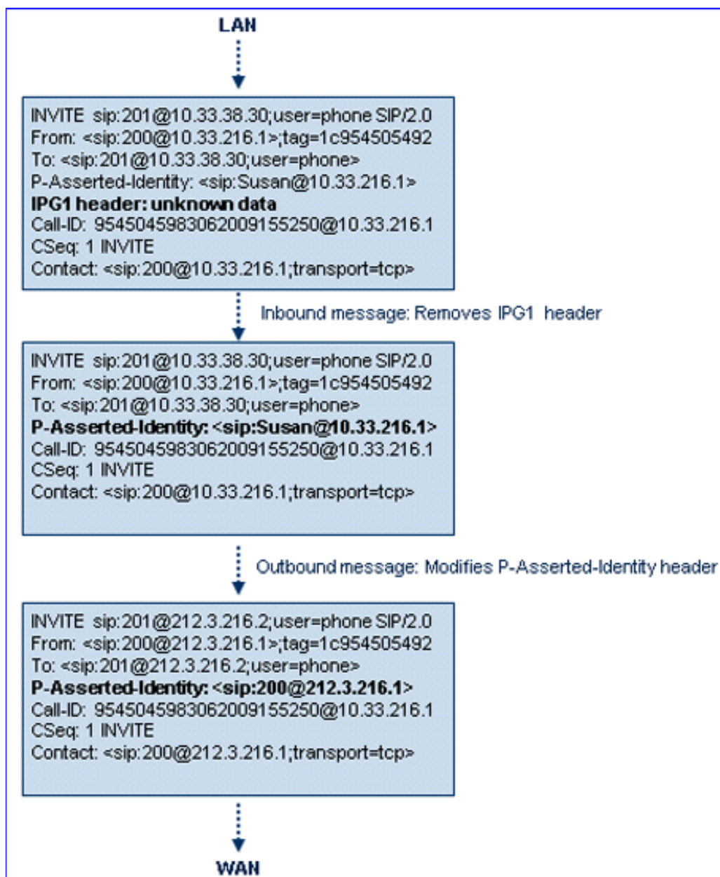
Figure 43-8: SBC Message Manipulation
