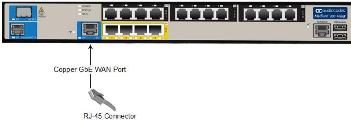
Figure 10: Cabling WAN Copper GE Port – Mediant 800C MSBR
