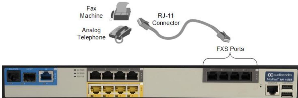
2. Connect the other end of the cable to the required telephone interface (e.g., fax machine, dial-up modem, and analog POTS telephone).
