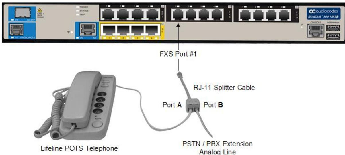
Figure 29: Cabling FXS Lifeline – Mediant 800C MSBR
