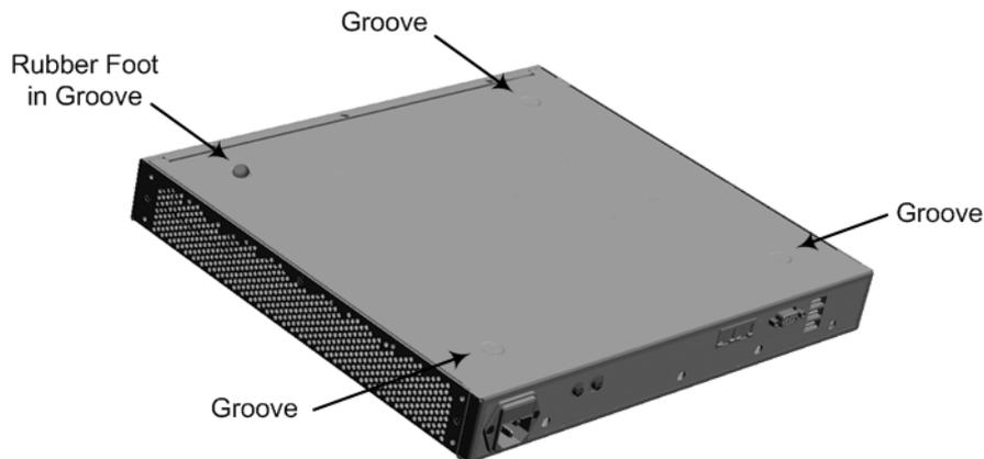
4. Flip the device over again so that it rests on the rubber feet and place it in the required position on a desktop.
