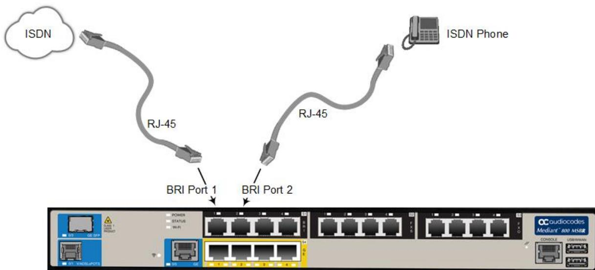
**Figure 34: Cabling BRI PSTN Fallback – Mediant 800C MSBR**
