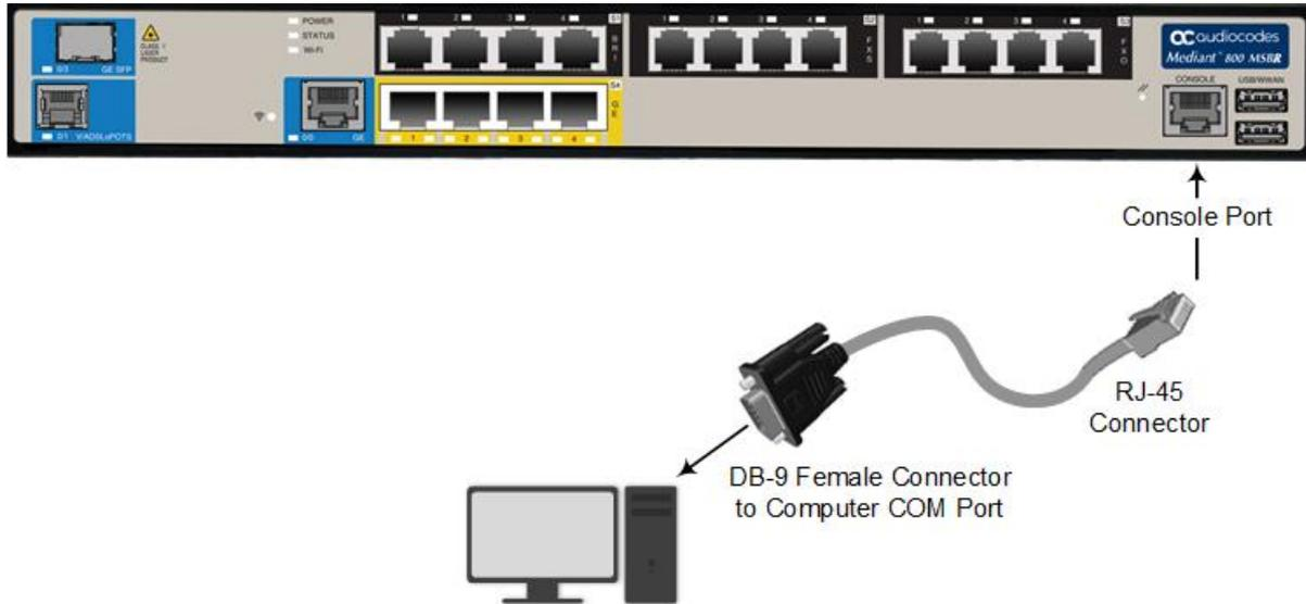
**Figure 40: Cabling Serial Interface - Mediant 800C MSBR**
