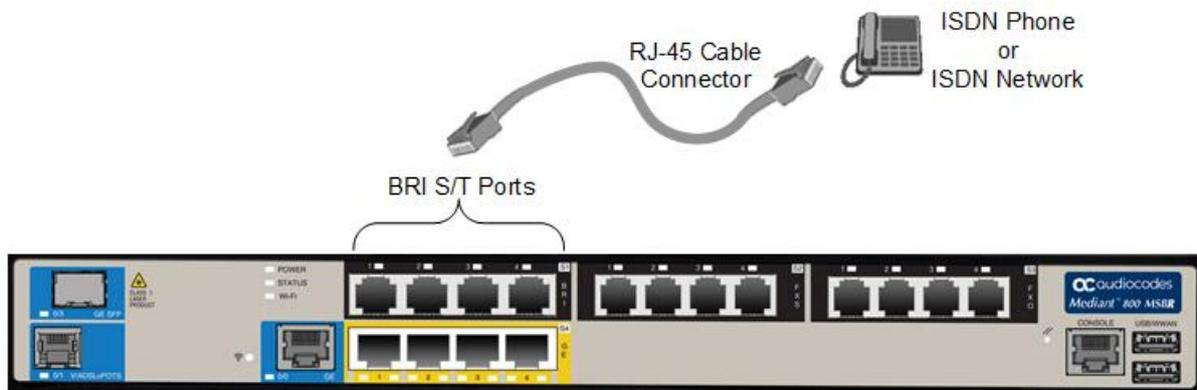
**Figure 32: Cabling BRI Ports – Mediant 800C MSBR**
