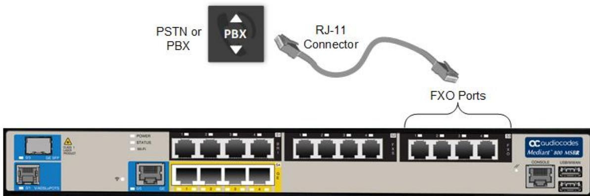
2. Connect the other end of the cable to the required telephone interface: (e.g., telephone exchange analog lines or PBX extensions).
