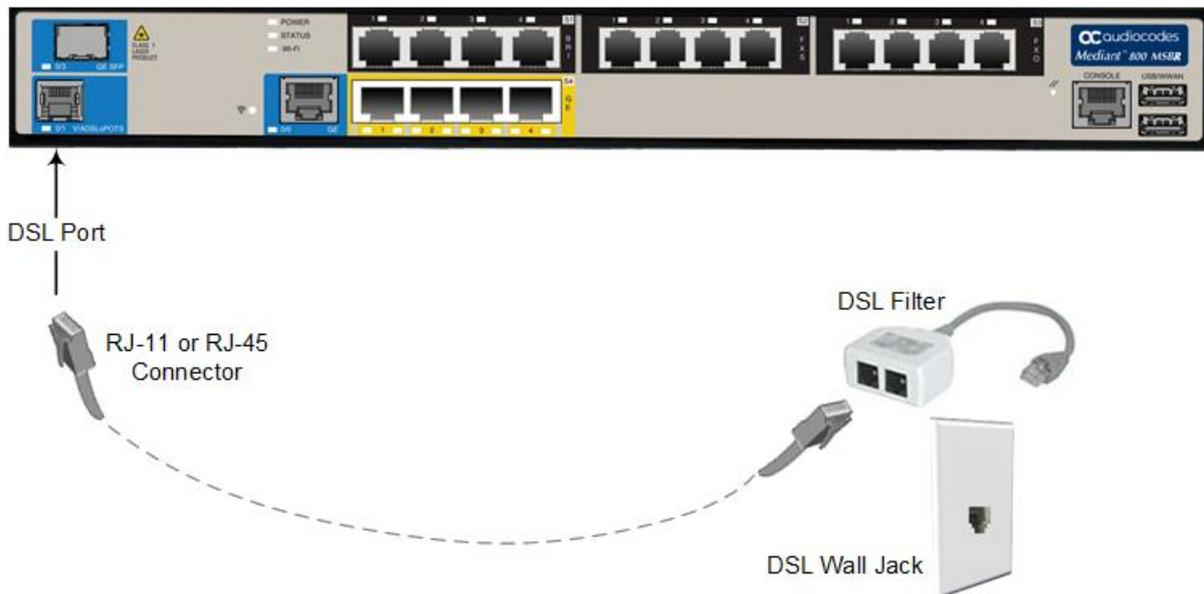
Figure 17: Cabling xDSL WAN Port – Mediant 800C MSBR
