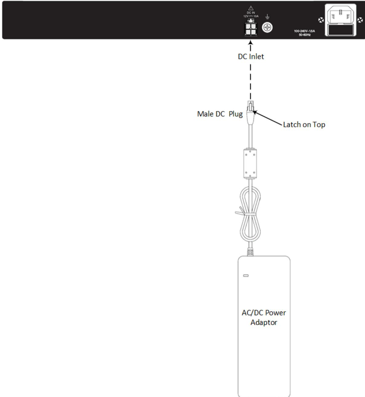
2. Plug the female connector that is located on one end of the AC power cord (supplied), into the AC/DC power adaptor.
