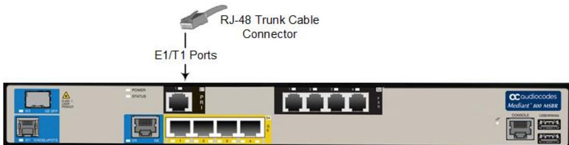
**Figure 37: Cabling E1/T1 Ports – Mediant 800C MSBR**
