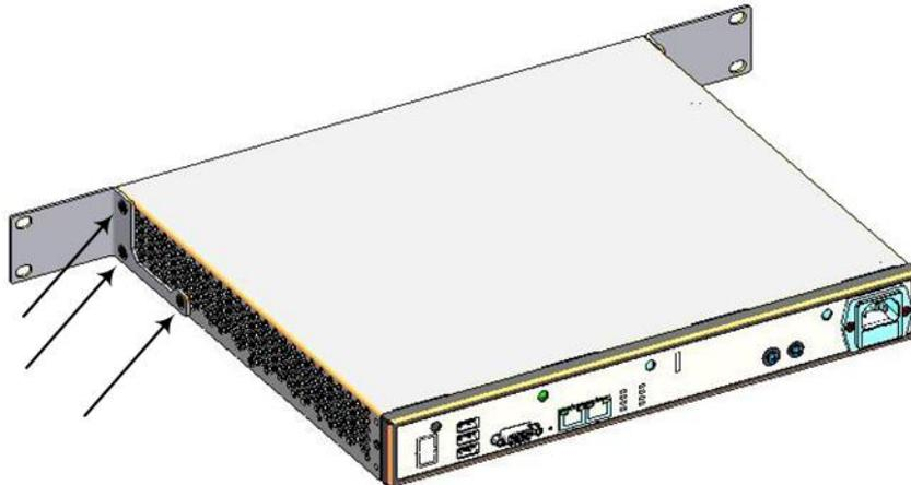
2. Place the device on a pre-installed shelf in the rack.
