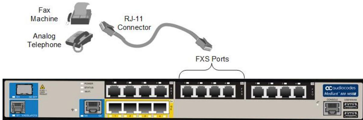
**Figure 24: Connecting FXS Interfaces – Mediant 800C MSBR**
