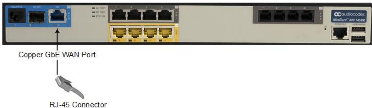
2. Connect the other end of the cable to the Ethernet WAN (e.g., ADSL or Cable modem).
