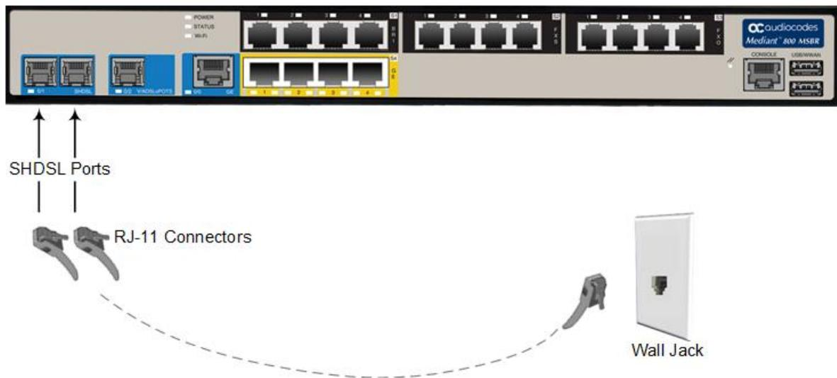
2. Connect the other end of the cable(s) to an RJ-11 wall jack.
