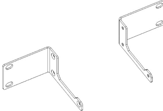
**To mount the device in a 19-inch rack using mounting brackets:**
