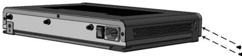
Figure 4-14: Attaching Bracket to Device using Side-Panel Screws
