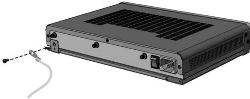
Figure 13: Attaching Bracket to Device using Ground Screw with Grounding Lug
