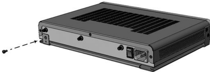
Figure 12: Attaching Bracket to Device using Grounding Screw
