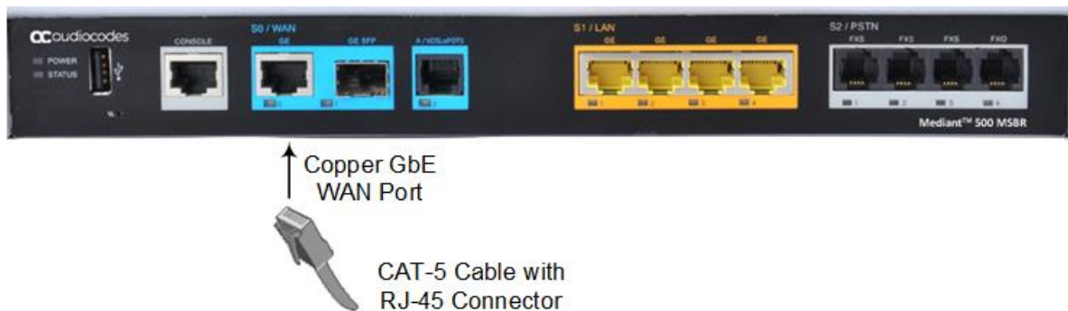
Figure 21: Cabling the WAN Copper GbE Port
