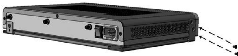
Figure 4-14: Attaching Bracket to Device using Side-Panel Screws
