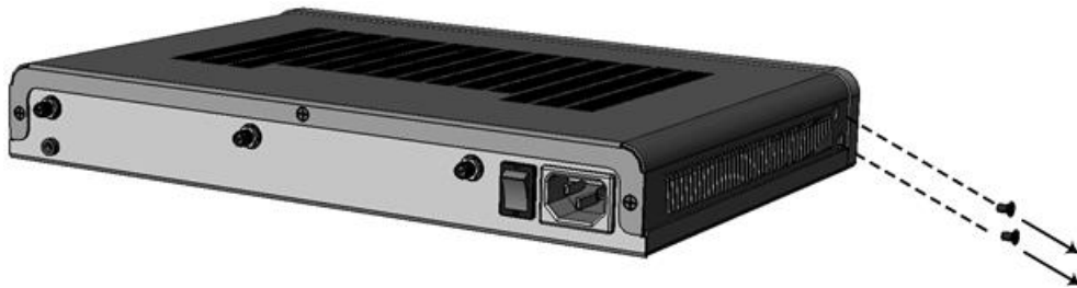
Figure 9: Removing Side-Panel Screws
