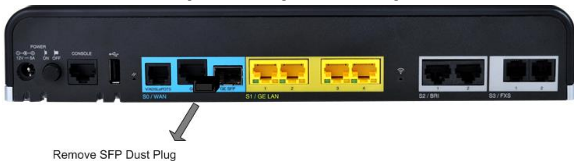
Figure 11: Removing Protective Dust Plug
