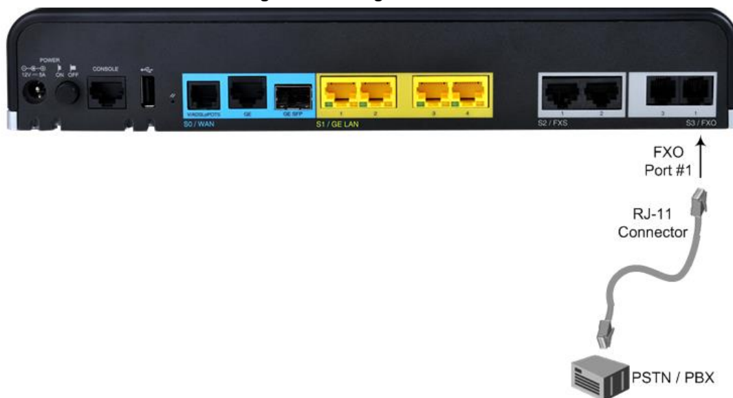
Figure 23: Cabling FXO Interfaces
