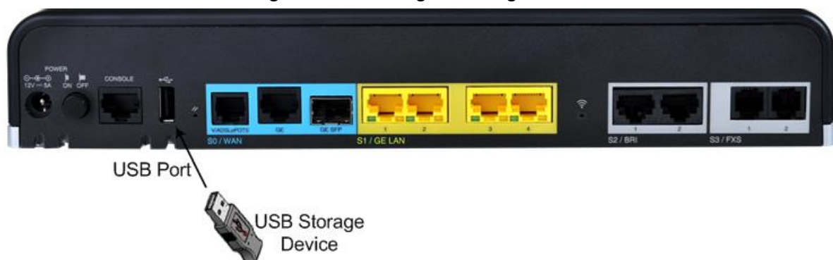
Figure 27: Connecting USB Storage Device
