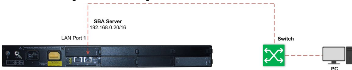
Figure 8-3: Connecting OSN3B and OSN4 Module to Network
