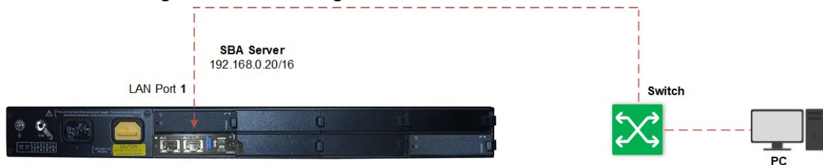
Figure 8-2: Connecting OSN3C and OSN4B Module to Network
