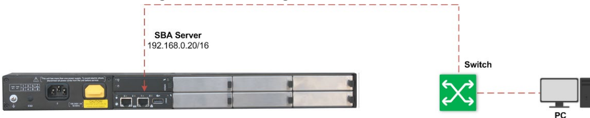
Figure 8-4: Connecting OSN3 Module to Network
