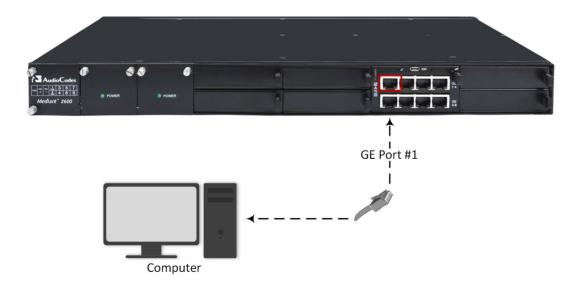
2. Change the IP address of your computer to correspond with the device's default IP address and subnet mask.
