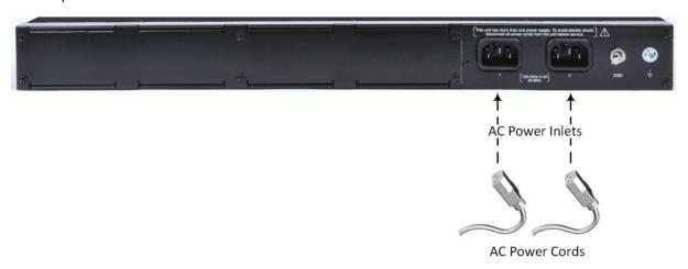
2. Connect the plug at the other end of the AC power cord to a standard electrical outlet.
