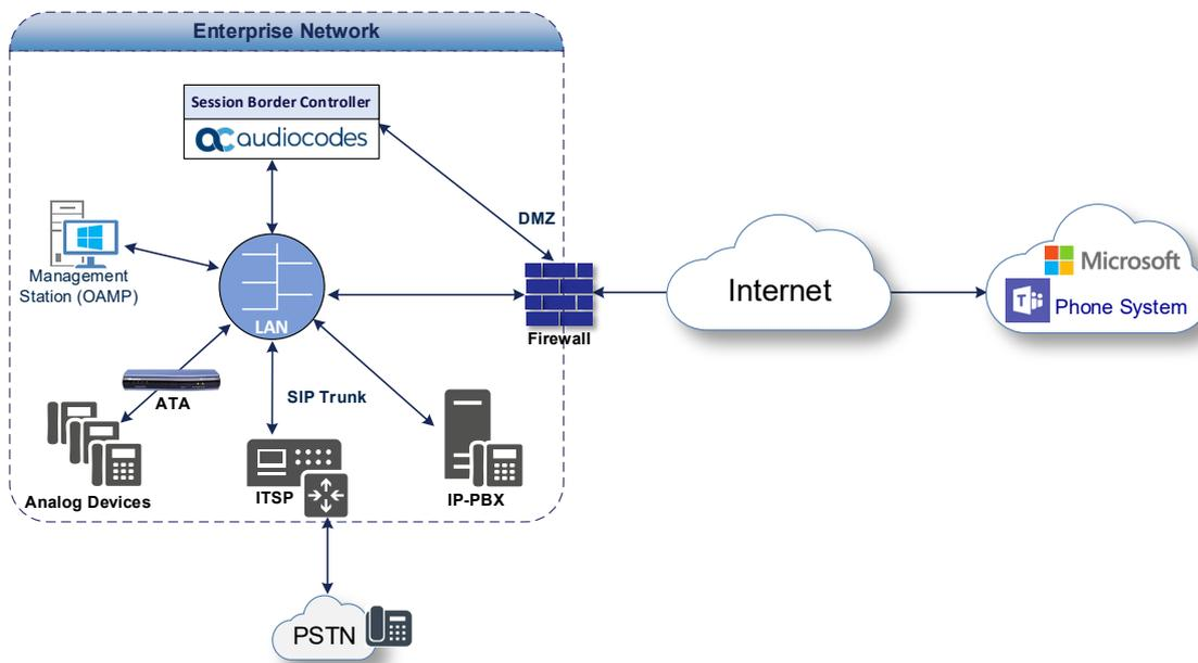
Figure 2-2: Connection Topology with SIP Trunk on the WAN
