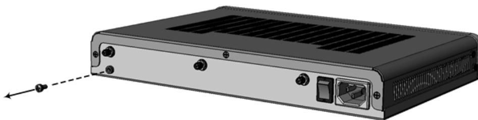
Figure 4-6: Removing Ground Screw
