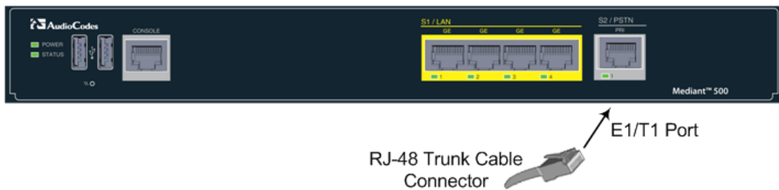
Figure 5-4: Cabling E1/T1 Port
