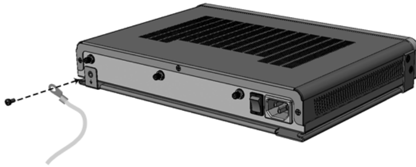
Figure 4-11: Attaching Bracket to Device using Ground Screw with Grounding Lug
