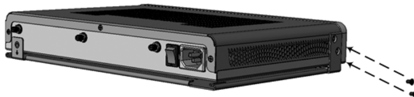
Figure 4-12: Attaching Bracket to Device using Side-Panel Screws
