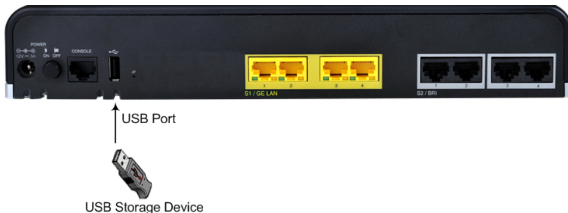
Figure 5-13: Connecting USB Storage Device
