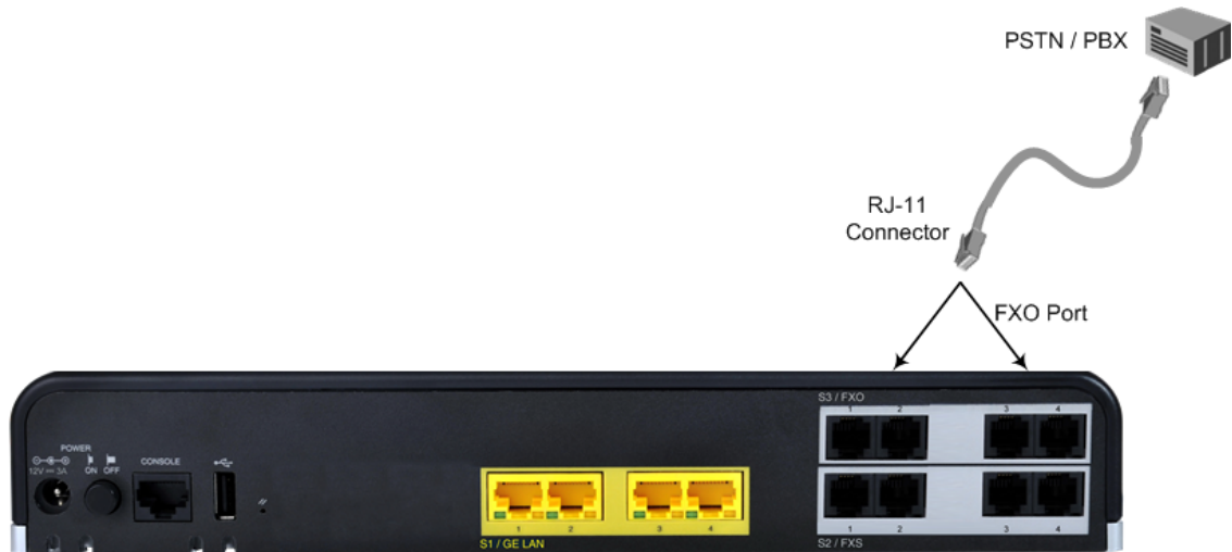
Figure 5-9: Connecting FXO Interfaces
