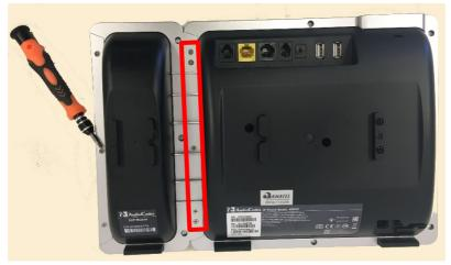
✓ Step 6: [Refer again to the figure above] Secure the connection of the two units by screwing in these five screws.
