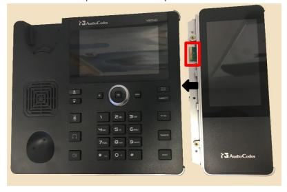
✓ Step 4: Attach the panel that you removed from the phone in Step 3 to the side of the Expansion Module, like this:
