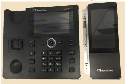
✓ Step 2: Invert the phone on a surface that won't scratch the screen such as a towel or printer paper. Avoid inverting the phone on the surface of a desk. Then unscrew the three screws shown below in order to remove the phone's side panel:
