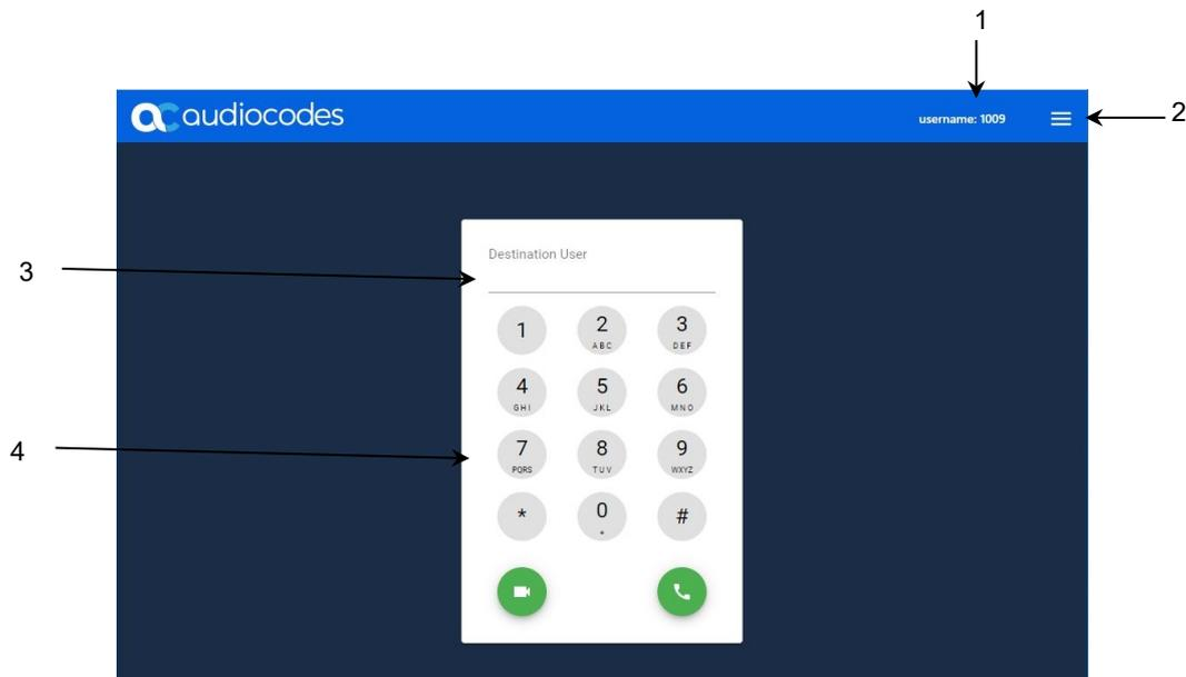
**Figure 3-4: Description of Main Page (Dialpad) of WebRTC Softphone Client**
