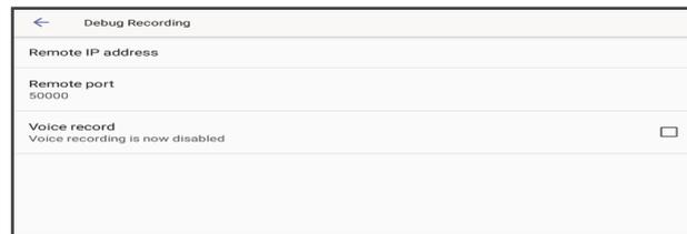
4. Configure the remote IP address and port.
