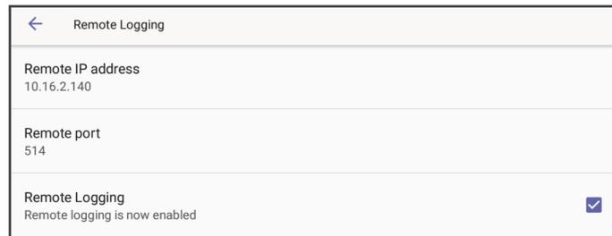
4. Configure the 'Remote IP address' and 'Remote port' and enable 'Remote Logging'; the device starts sending logs to the Syslog server.
