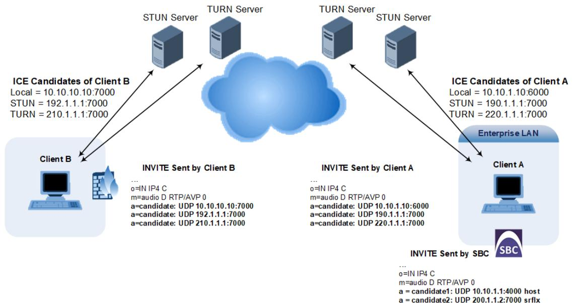
To support ICE, the device's leg interfacing with the ICE-enabled client (SIP entity) must be enabled for ICE. This is done by using the IP Profile parameter 'ICE Mode' (see [Configuring IP Profiles](#)), which can be configured to **Lite** or **Full**.
