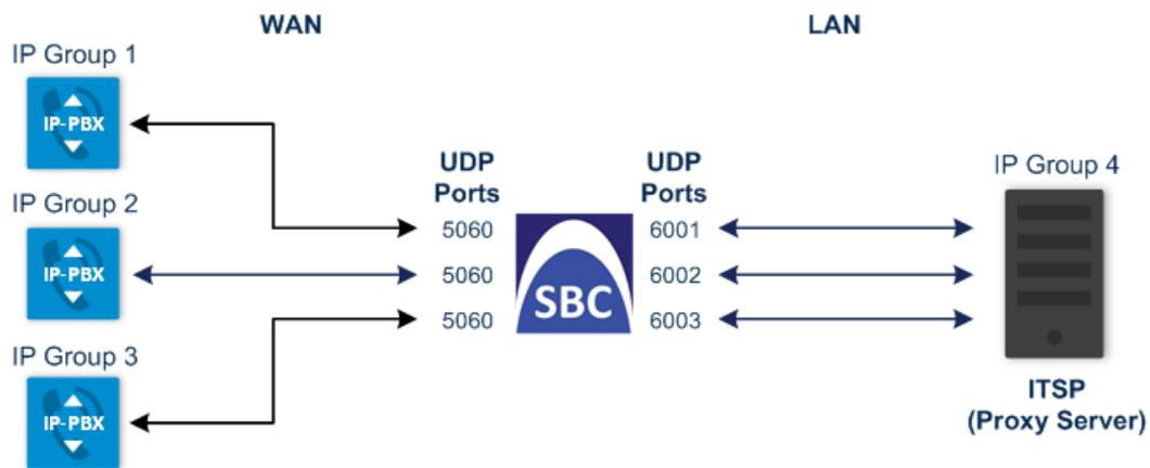
For each IP PBX, the device sends SIP messages to the proxy server using the specific local, UDP port on the leg interfacing with the proxy server. For SIP messages received from the proxy server, the device routes the messages to the appropriate IP PBX according to the local UDP port on which the message was received. On the leg interfacing with the IP PBXs, the device uses the same local UDP port (e.g., 5060) for all IP PBXs (send and receive).
