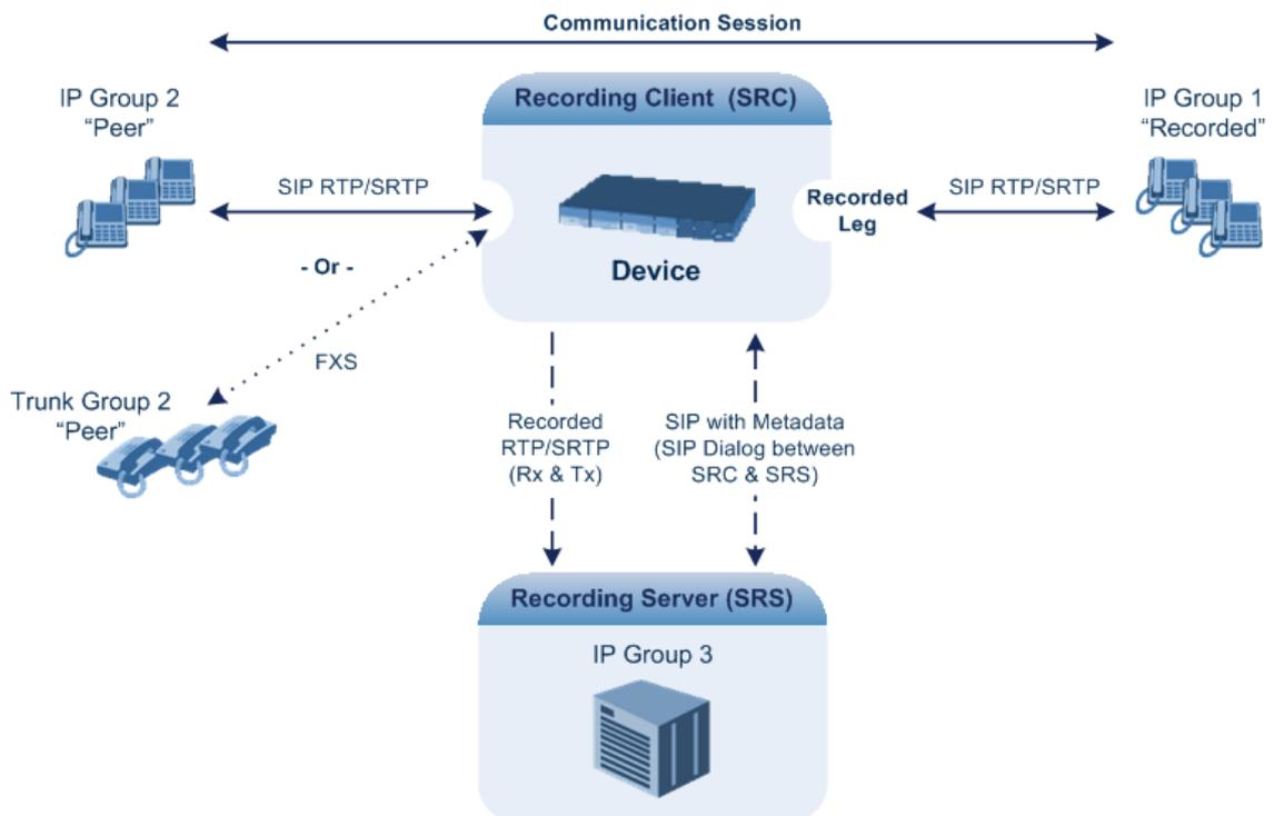
The device can record calls between two IP Groups, or between an IP Group and a Trunk Group for Gateway calls. The type of calls to record can be specified by source and/or destination prefix number or SIP Request-URI, as well as by call initiator. The side ("leg") on which the recording is done must be specified. Specifying the leg is important as it determines the various call media attributes of the recorded RTP (or SRTP) such as coder type.
