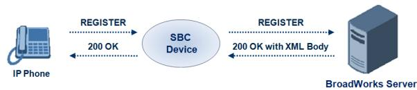
The device saves the users in its registration database with their phone numbers and extensions, enabling future routing to these destinations during survivability mode when communication with the BroadWorks server is lost. When in survivability mode, the device routes the call to the Contact associated with the dialed phone number or extension number in the registration database.
