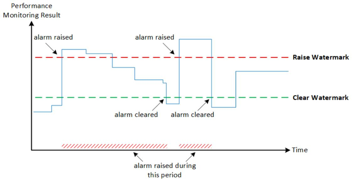
As shown in the illustration, the alarm is only raised once it crosses the *raise watermark* threshold in the up direction (i.e., performance monitoring parameter value is greater than the threshold). The raised alarm is only cleared when it crosses the clear watermark threshold.
