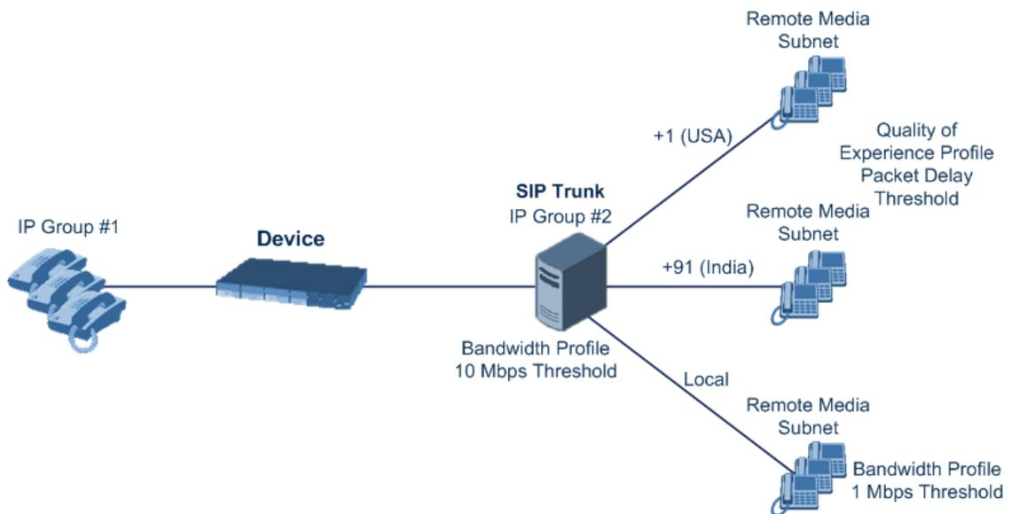
The following procedure describes how to configure Remote Media Subnets through the Web interface. You can also configure it through ini file [RemoteMediaSubnet] or CLI (`configure voip > remote-media-subnet`).
