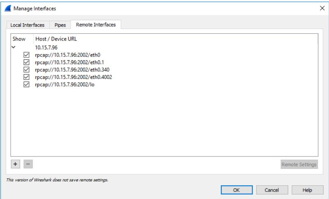
The 'Manage Interfaces' dialog box shows the 'Remote Interfaces' tab with a list of interfaces for host 10.15.7.96. All checkboxes are selected.
