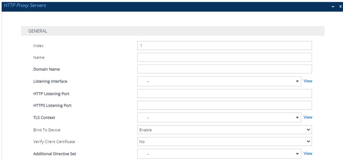
4. Configure an HTTP Proxy server according to the parameters described in the table below.
