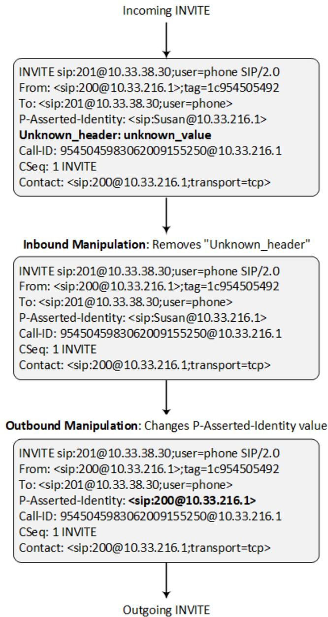
This manipulation example is done by configuring two Message Manipulation rules, where Rule #1 is assigned to the source IP Group and Rule #2 to the destination IP Group.
