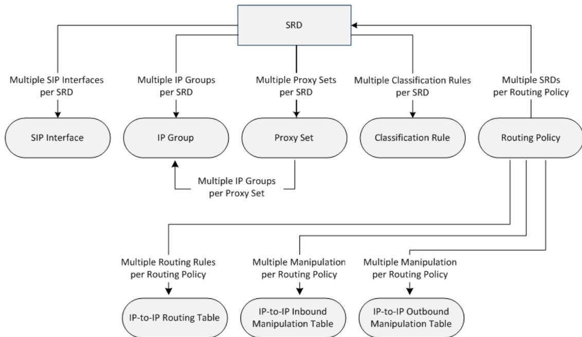
The main configuration entities and their involvement in the call processing is summarized in following figure. The figure is used only as an example to provide basic understanding of the configuration terminology. Depending on configuration and network topology, the call process may include additional stages or a different order of stages.
