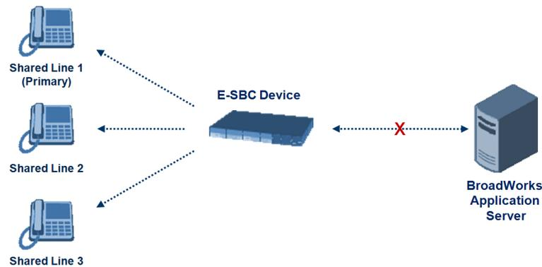
To configure this capability, you need to configure a shared-line, inbound manipulation rule for registration requests to change the destination number of the secondary extension numbers (e.g. 601 and 602) to the primary extension (e.g., 600). Call forking must also be enabled. The following procedure describes the main configuration required.
