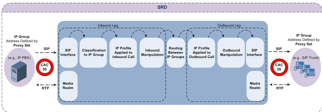
1. The device determines the SIP Interface on which the incoming SIP dialog is received and thus, determines its associated SRD.
