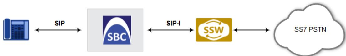
For the interworking process, the device maps between ISUP data (including cause codes) and SIP headers. For example, the E.164 number in the Request-URI of the outgoing SIP INVITE is mapped to the Called Party Number parameter of the IAM message, and the From header of the outgoing INVITE is mapped to the Calling Party Number parameter of the IAM message.
