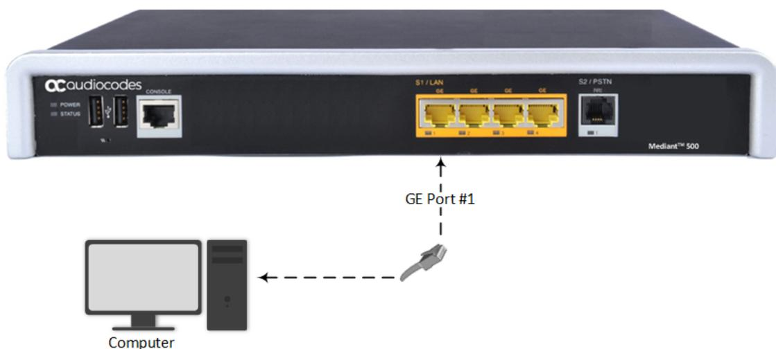
2. Change the IP settings of your computer to correspond with the default OAMP IP address and subnet mask of the device.
