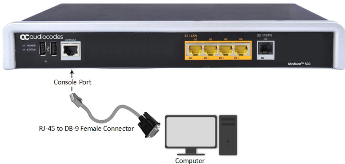
2. Establish serial communication with the device using a terminal emulator program such as HyperTerminal, with the following communication port settings:
