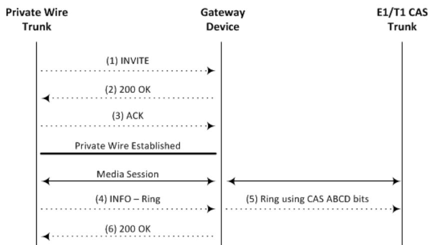
The following is an example of the message flow for interworking private wire Hook Switch states between the private wire trunk and the E1/T1 CAS trunk:
