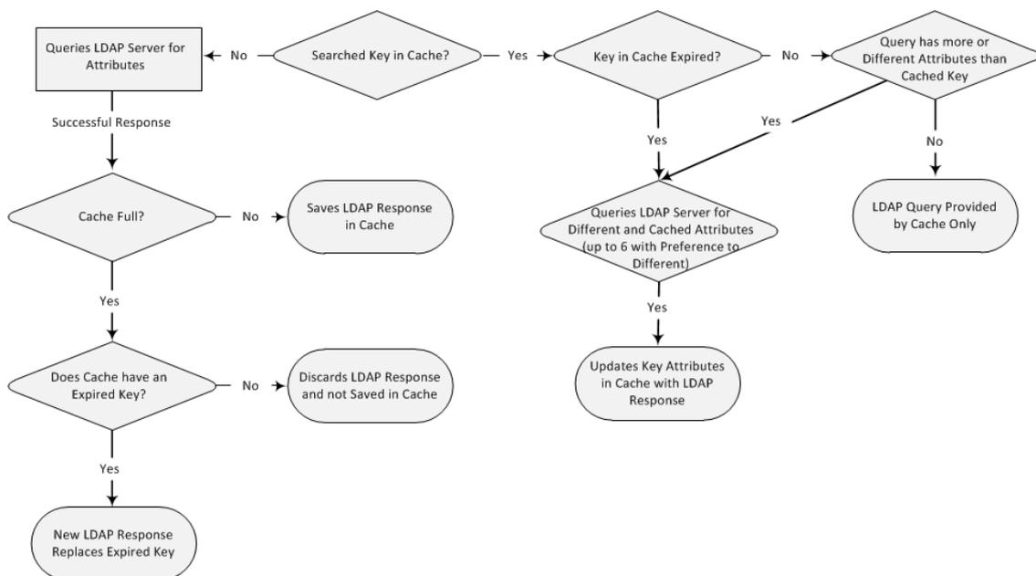
If an LDAP query is required for an Attribute of a key that is already cached with that same Attribute, instead of sending a query to the LDAP server, the device uses the cache. However, if an LDAP query is required for an Attribute that doesn't appear for the cached key, the device queries the LDAP server, and then saves the new Attribute (and response) in the cache for that key.
