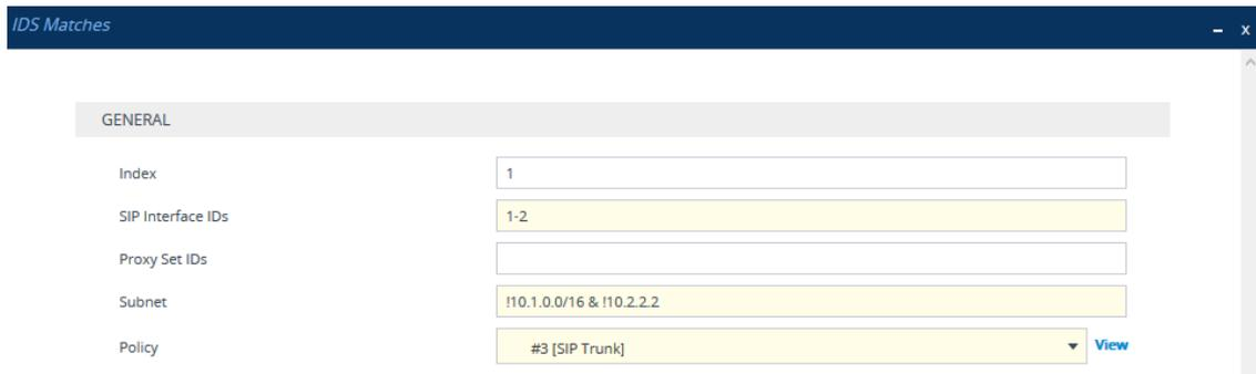
The figure above shows a configuration example where the IDS Policy "SIP Trunk" is applied to SIP Interfaces 1 and 2, and to all source IP addresses outside of subnet 10.1.0.0/16 and IP address 10.2.2.2.
