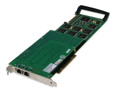
The **SmartWORKS™ PCM** series cards have been designed to combine the same features and capabilities of SmartWORKS cards with a PCM32 front end. This board has been designed to work with the PCM32 Megalink protocol.
