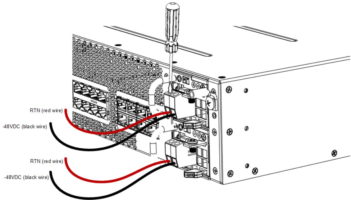
8. Connect the DC power leads to a 48-VDC power source.
