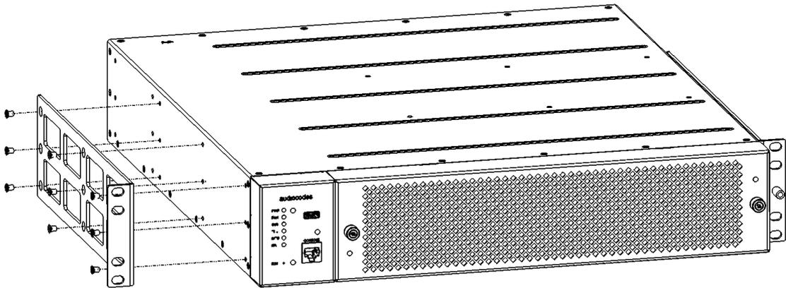
3. Place the chassis onto the shelf that you installed in the 19-inch rack (see Step 1).
