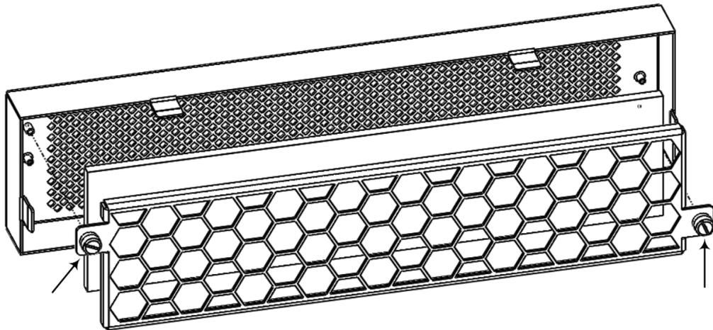
3. Pull out the exposed air filter from the enclosure of the Air Filter cover and dispose of it:
