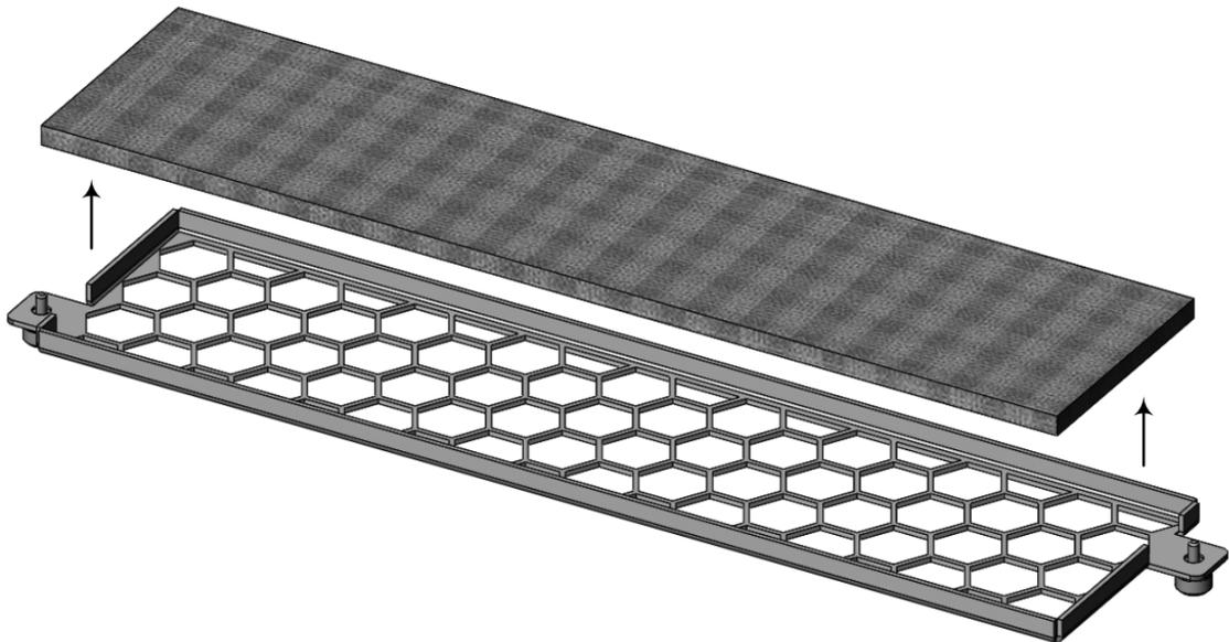
4. Insert the new filter into the enclosure of the Air Filter cover.
