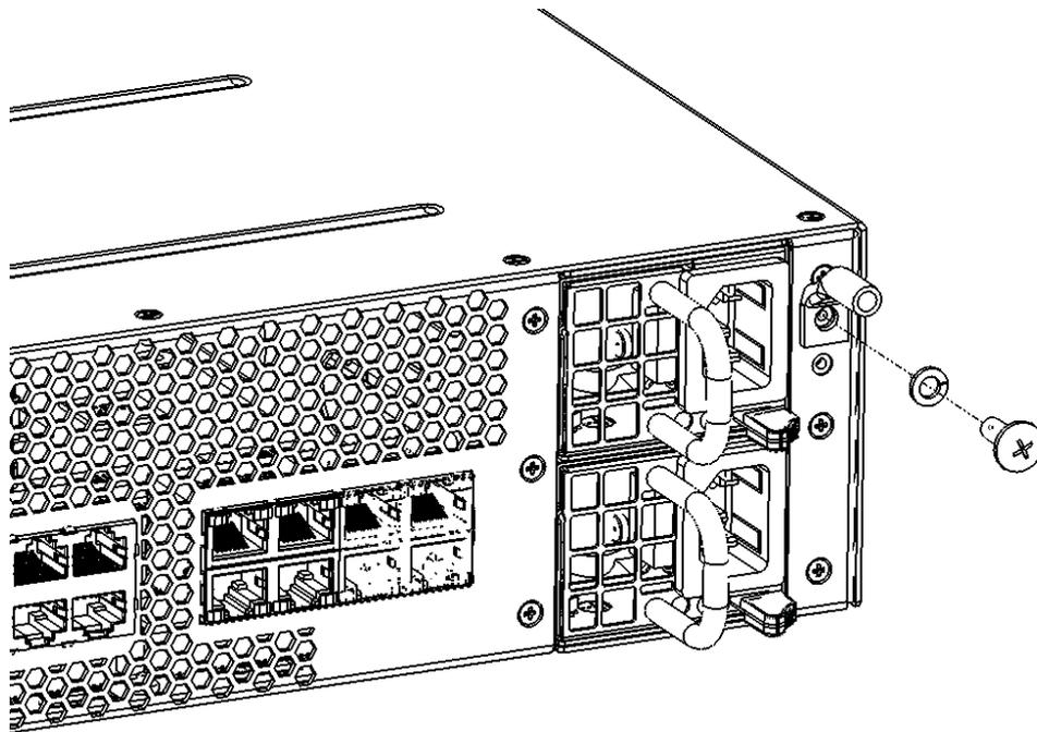
4. Connect the other end of the grounding wire to the building's protective earth. This should be in accordance with the regulations enforced in the country in which the device is being installed.
