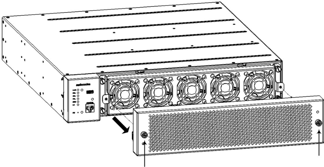
2. Remove the Air Filter cover, located on the inside of the Fan Tray cover, by removing the two flat-head, spring-loaded captive screws located on either side of the Air Filter cover, using a flathead screwdriver:
