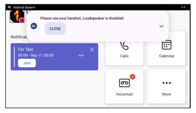
If after the feature is enabled, the user presses the 'Accept' softkey or the speaker hard key, the following popup message is displayed:
