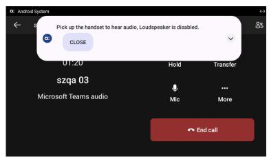
The user can then answer by picking up the handset or using a headset if a USB headset is connected. The popup indication then disappears.
