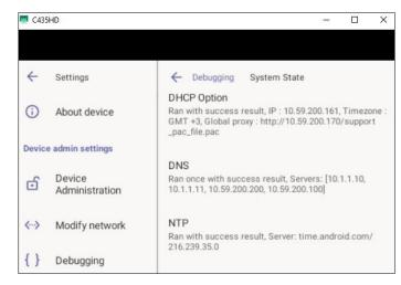
AudioCodes Android devices can configure VLAN via a DHCP Option when CDP/LLDP isn't allowed in the organization. The following DHCP Options offer a VLAN ID: Option 43, 132, 128, 129, 144, 157, 191. If the device gets more than one of these, it applies only one according to the aforementioned order of priority.
