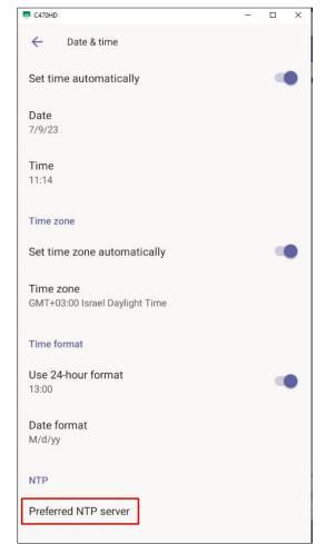
Admins can alternatively use the newly added parameter date\_time/ntp/server\_address in the phone's .cfg configuration file.
