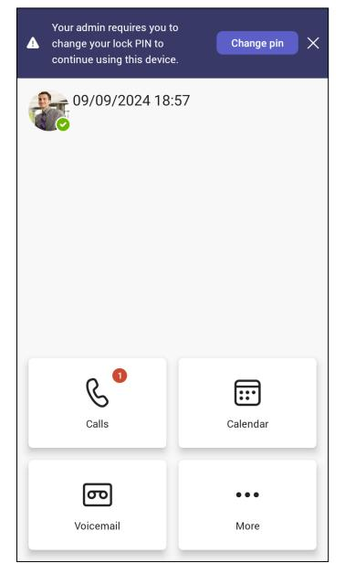
The configuration option is received as part of the configuration profile settings assigned to the device from Teams Admin Center. Once the timeout configured by admin lapses, the firmware locks the device.
