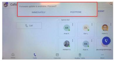
When any update is pushed to the device, the device's firmware detects whether the user is actively using the device. After determining this, an appropriate message and options are provided for the user to either delay the update or apply it immediately.
