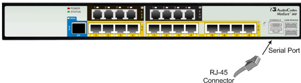
Figure 5-16: Cabling Serial Interface (RJ-45) on Mediant 800B
