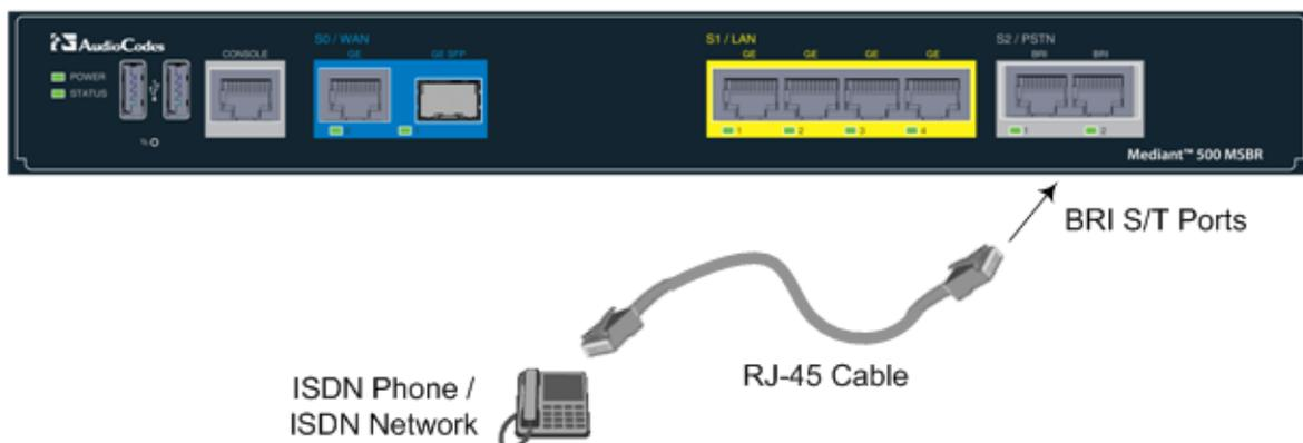
2. Connect the other end of the cable to your ISDN telephone or PBX/PSTN switch.
