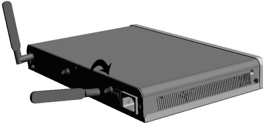
2. Orient the antennas as desired for optimal wireless performance. The antenna can be orientated in the vertical and horizontal planes. For best performance, it is recommended that the antennas be perpendicular (90 degrees) to the floor. In other words, orient the antennas straight up.
