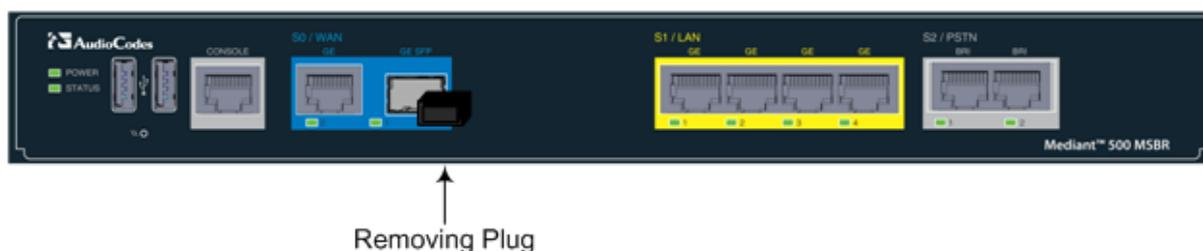
2. Connect a cable with LC-type plugs to the SFP transceivers (labeled **GE SFP**).
