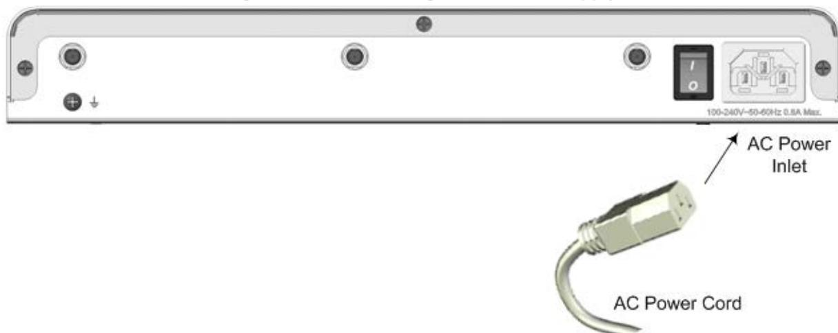
2. Connect the plug at the other end of the AC power cord to a standard electrical outlet.
