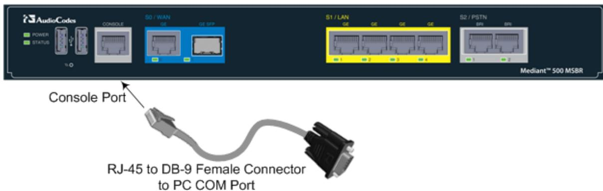
2. Connect the other end of the cable providing the 9-pin DB connector to the COM RS-232 communication port on your computer.
