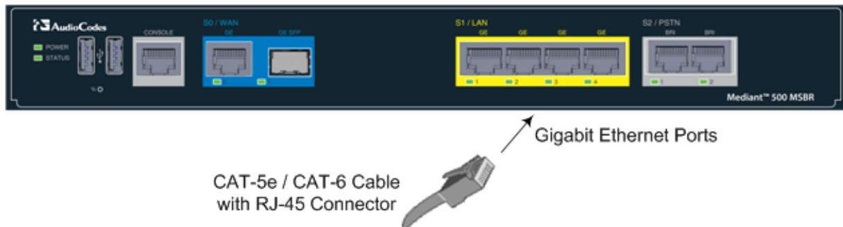
2. Connect the other end of the cable to the Gigabit Ethernet network.
