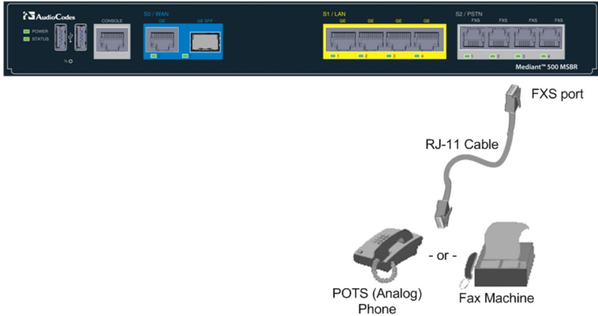
2. Connect the other end of the cable to the required telephone interface (e.g., fax machine, dial-up modem, or analog POTS telephone).
