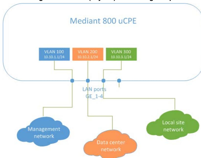
The Mediant 800 uCPE’s MSBR module is used as Layer 2 switch. Three VLAN’s are created:
