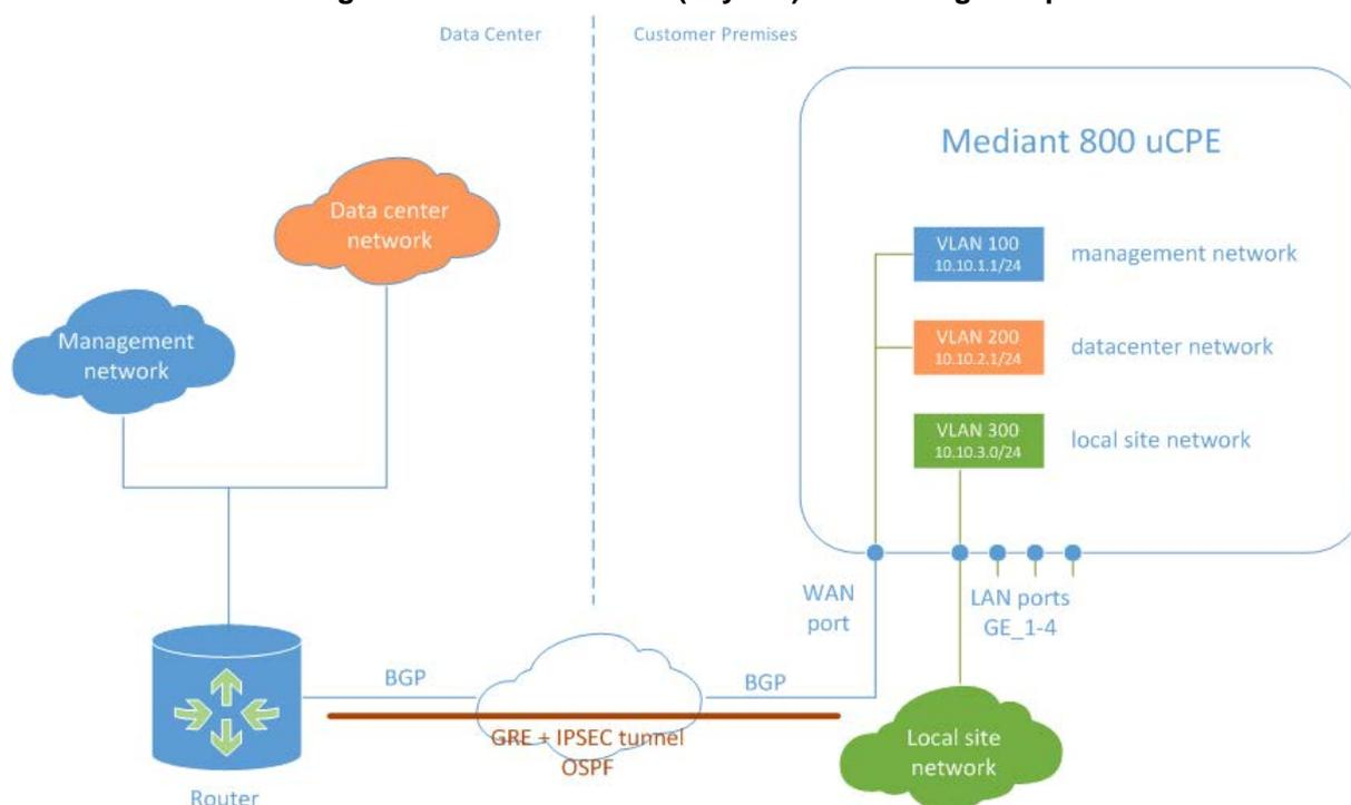
We use the same three VLANs – 100, 200 and 300 – as in the previous networking setup (described in Section 06.2), to connect the Mediant 800 uCPE to management, Datacenter and local site networks correspondingly.
