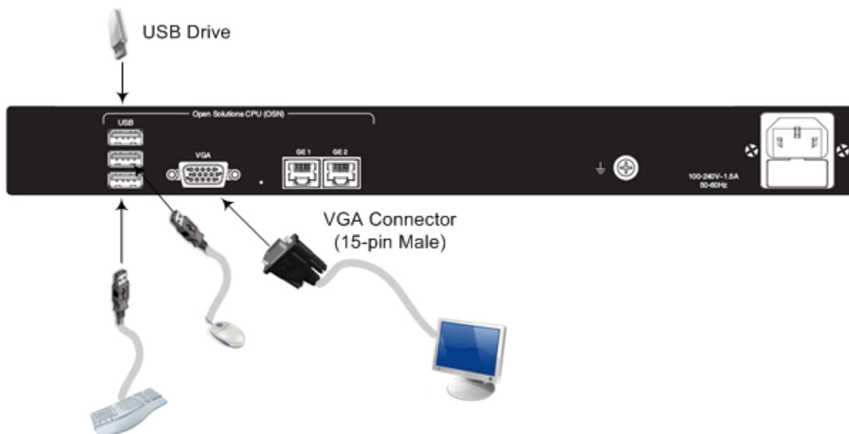
2. Insert the installation USB drive into the OSN module.
