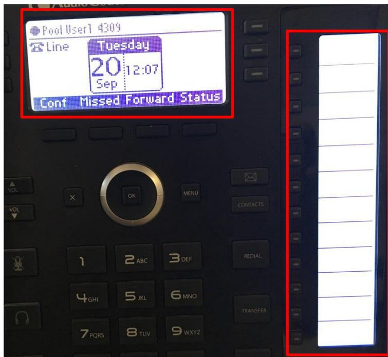
The figure above shows the phone screen (in idle mode) and sidecar (BLF keys and fields) of a phone in the pool.
