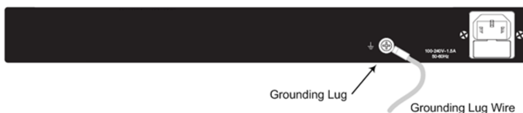
Figure 2-14: Grounding the Device
