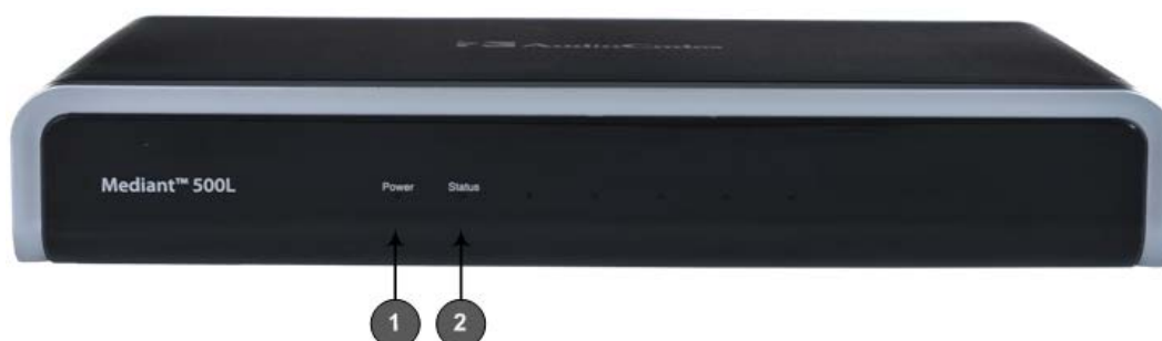
Figure 2-1: Front Panel - LEDs
