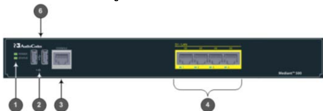
Figure 2-7: Front Panel - Ports
