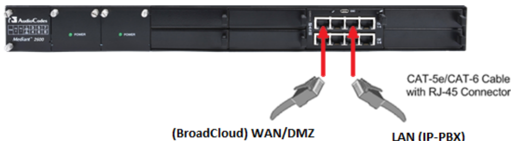
Figure 2-20: Connecting the LAN Ports
