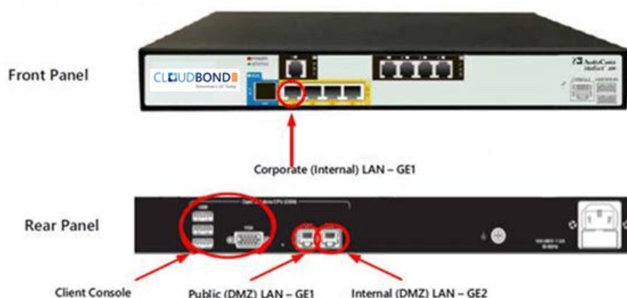
Figure 14-2: Utilizing the Second Ethernet Port on the CloudBond 365 Rear Panel
