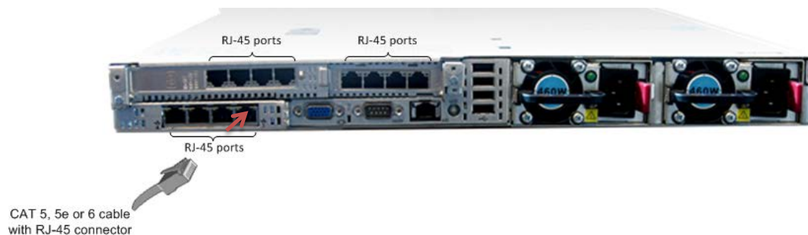
Figure 10-15: Connecting the Device to the IP Network
