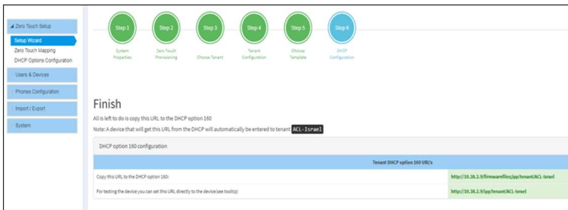
Figure 4-7: Step 6 – DHCP Configuration
